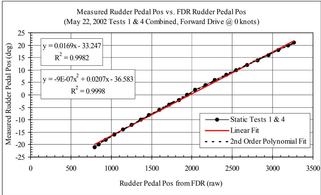
Graph 2: May 22, 2003 Rudder Pedal Test
