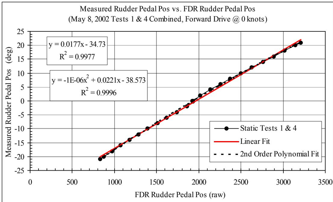
Graph 1: May 8, 2002 Rudder Pedal Test
