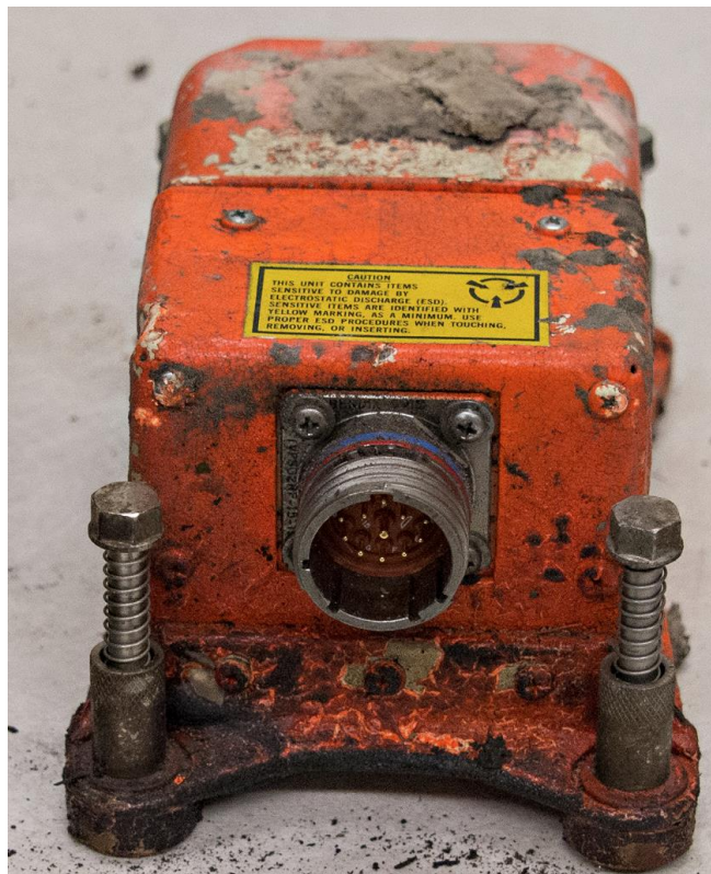
Figure 1. Damaged exterior of CSMU.
