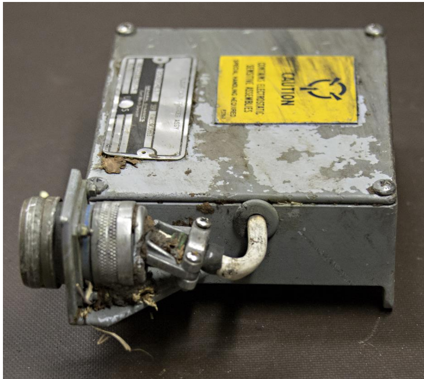
Figure 3. Damaged exterior of SDR.
