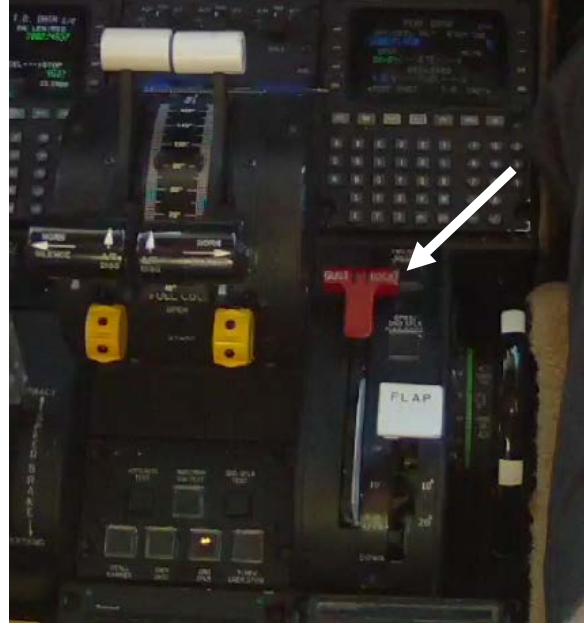
Figure 2. Gust lock handle in down/forward and latched (off) position
