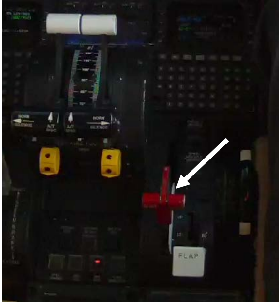
Figure 1. Gust lock handle in up/aft and latched (on) position.
