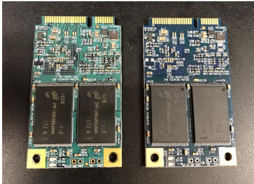
Figure 2. The NVM unit extracted from the processor unit. The NVM from the processor is shown on the left, the NVM from the dialer is shown on the right.
