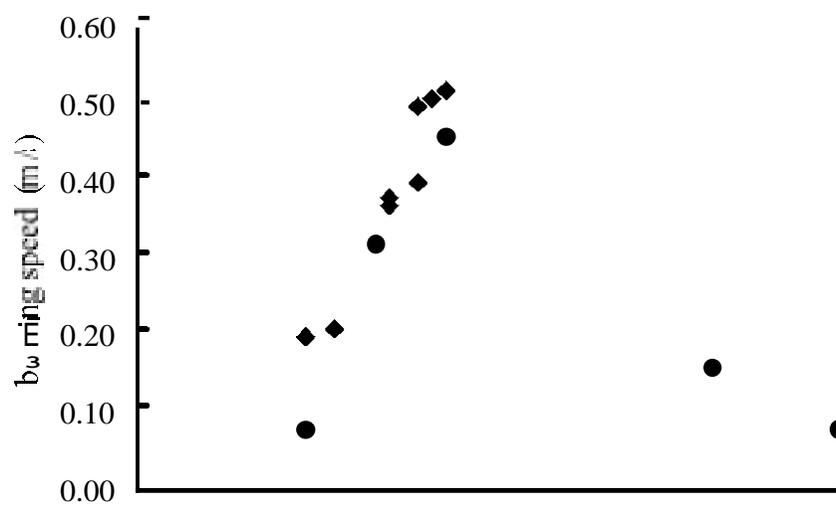
Figure 20: Effective burning speeds estimated from the pressure-time histories for hexane-air mixtures, initial pressure 1 atm, initial temperature 295 K.
