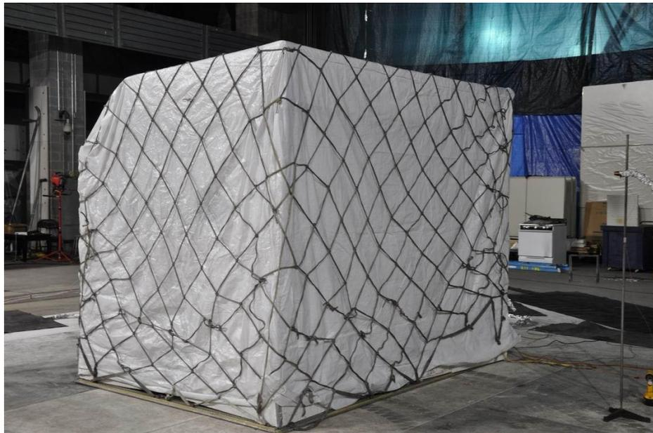
Figure 20: DMZ type container with plastic rain cover and cargo net
