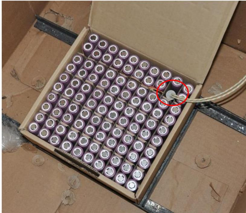
Figure 12: Box of batteries with cartridge heater in place (circled in red)
