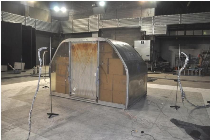
Figure 16: A2N type container with fuel load inside
