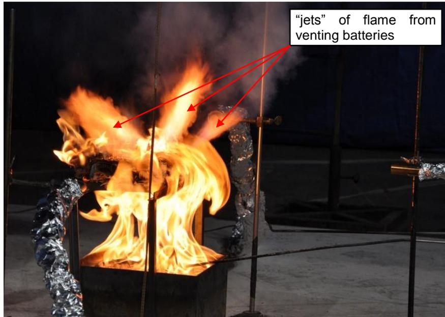
Figure 10: Box of lithium-ion batteries burning over propane burner exhibiting battery venting and electrolyte combustion
