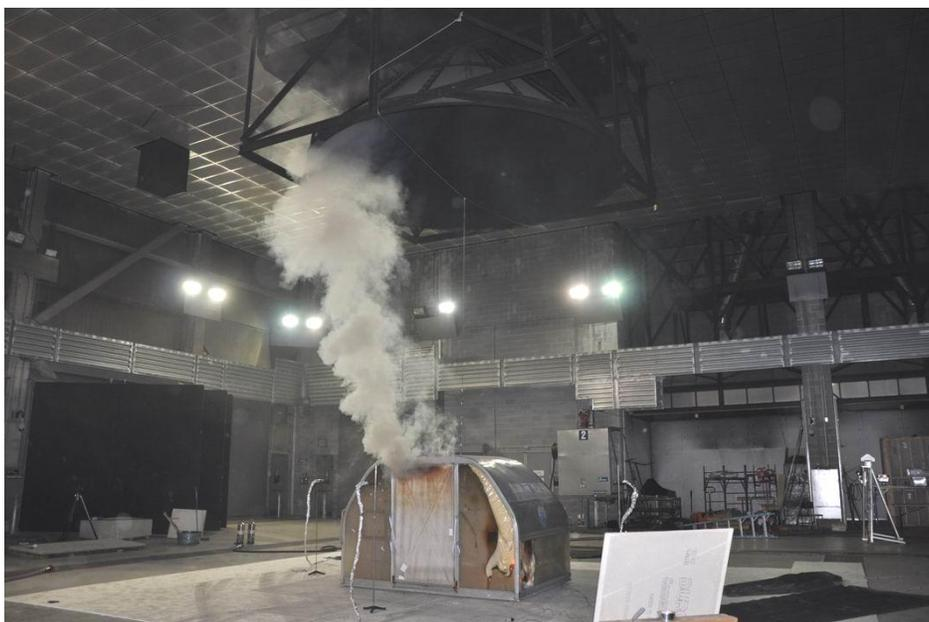
Figure 17: Smoke exiting above roll-up door on A2N type container
