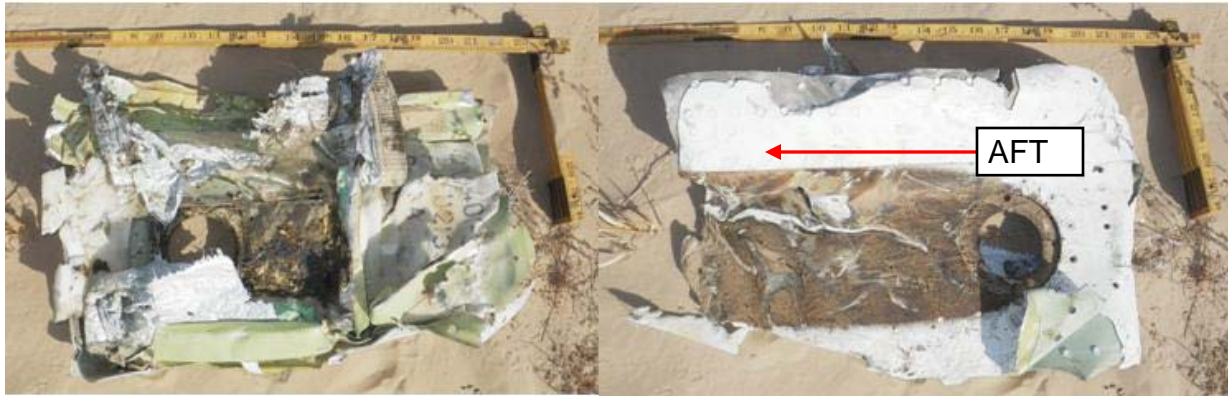
Figure 13: Fuselage skin piece with smoke shutter cutout (interior on the left, exterior on the right)
