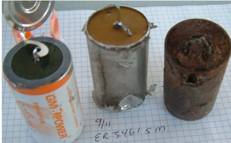
Figure 26: D-Cell size lithium primary batteries. Photo shows fire damaged and undamaged batteries
