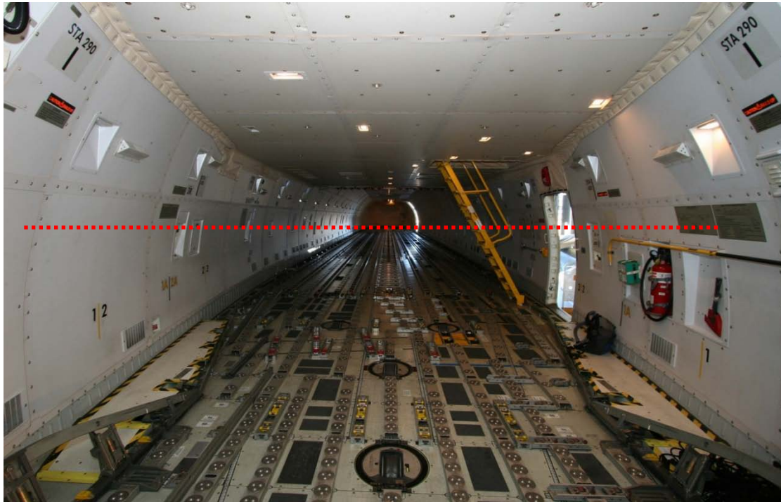
Figure 20: Exemplar interior showing stairs to the flight deck and a dotted line showing the level of the smoke layer
