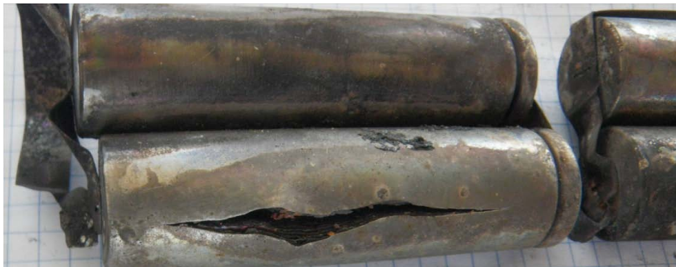
Figure 24: Fire damaged remains of battery pack with a fractured cell
