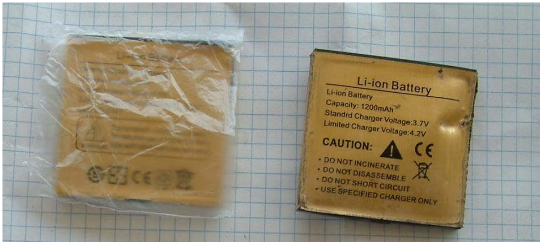
Figure 30: Lithium-ion, mobile phone type battery
