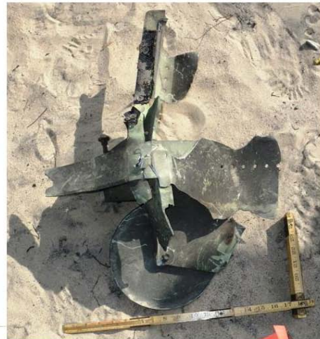
Figure 12: Structure piece with pulley (showing both sides)
