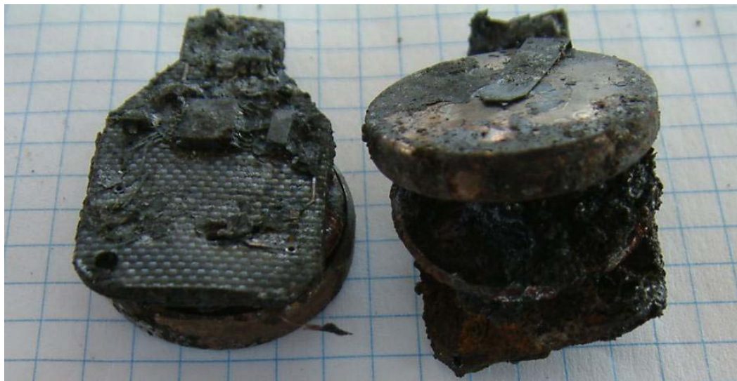
Figure 27: Lithium primary button sized flat cell batteries (watch style) with small circuit board
