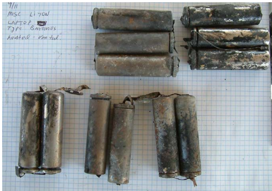
Figure 25: Additional battery pack remains
