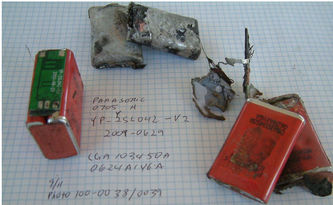
Figure 32: Intact and fire damaged Panasonic batteries (2-pack Li-ION set)
