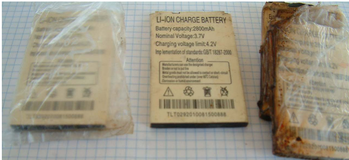
Figure 31: Lithium-ion, mobile phone type battery
