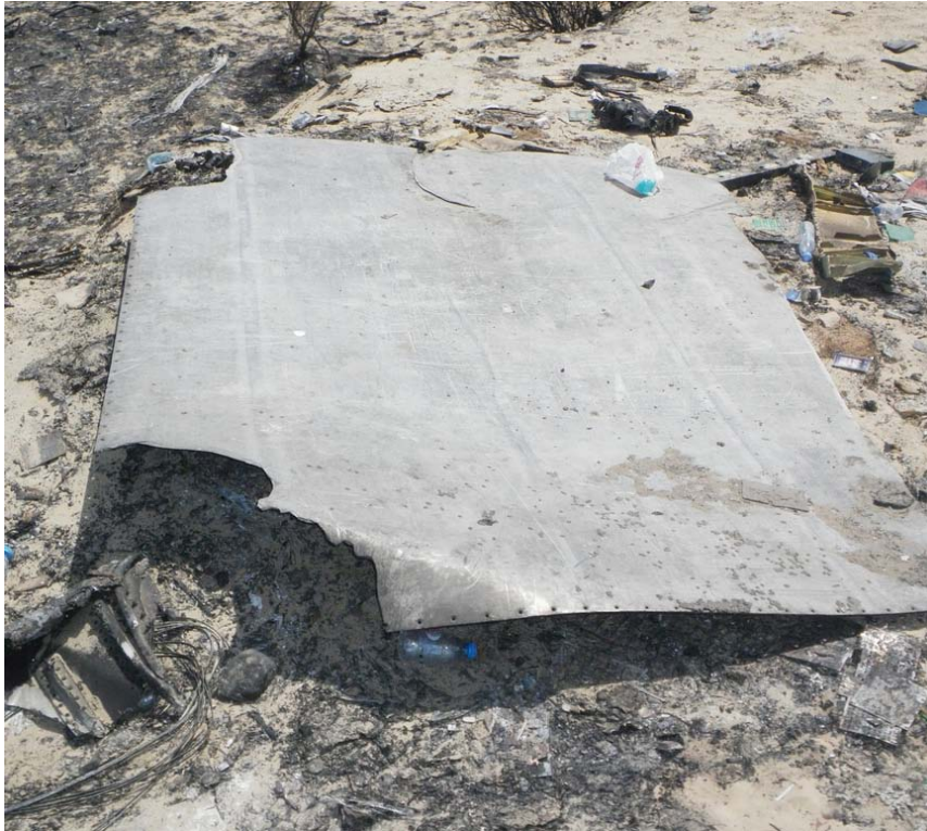
Figure 2: Cargo container base plate
