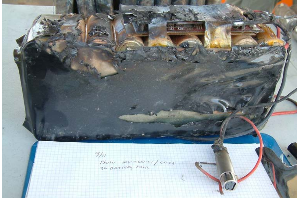
Figure 28: 36-cell lithium-ion battery pack with thermal damage.
