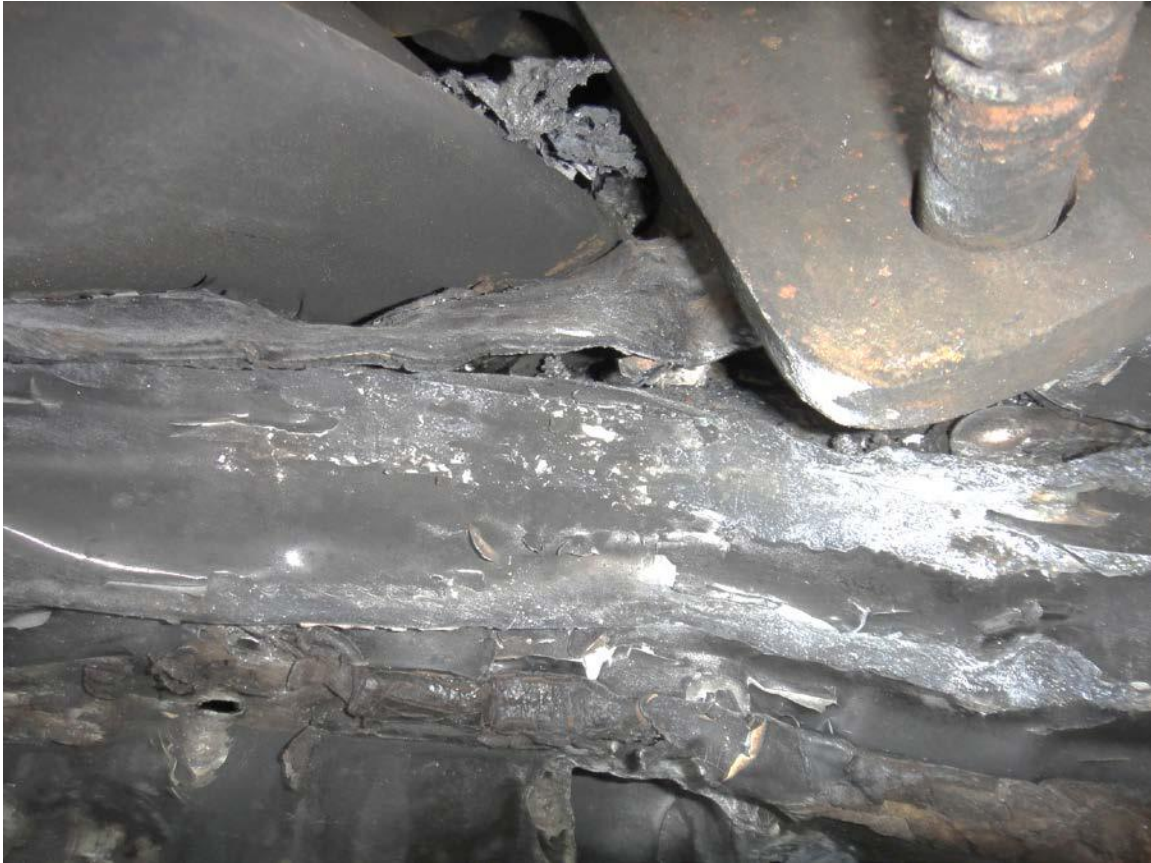
Figure 31. Close-up of erosion of SUV frame.
