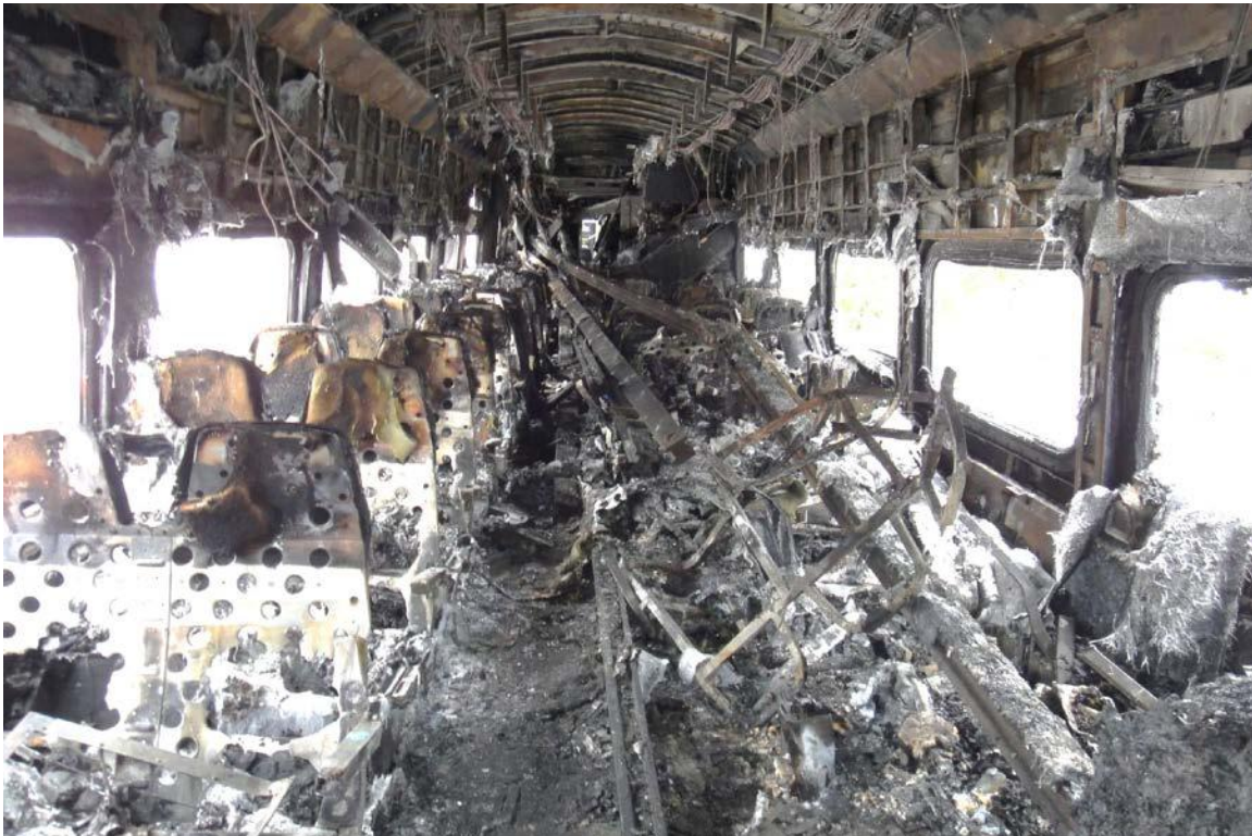
Figure 16. Passenger Compartment - Overall interior of MN 4333 at accident site.
