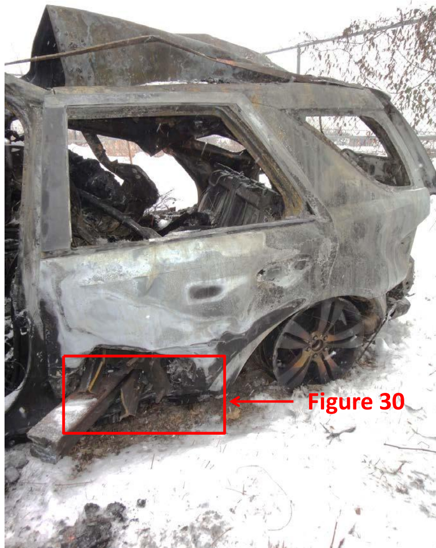
Figure 29. Entry point for 3rd rail into SUV.
