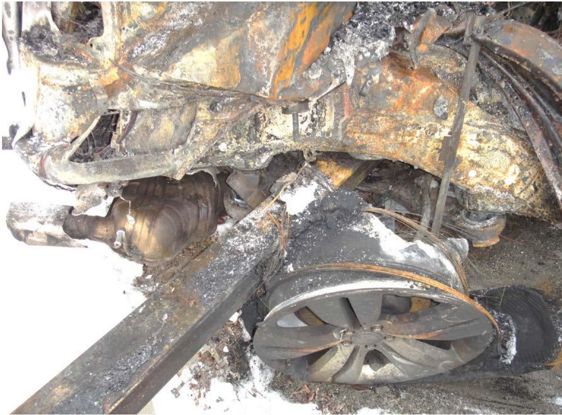
Figure 27. Rear passenger side tire with fire damaged rim.
