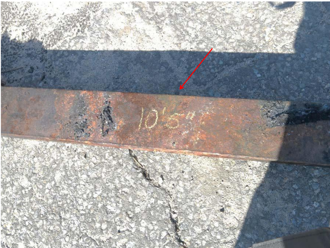
Figure 22. Localized thermal damage (highlighted with red arrow) to surface of rail removed from SUV.
