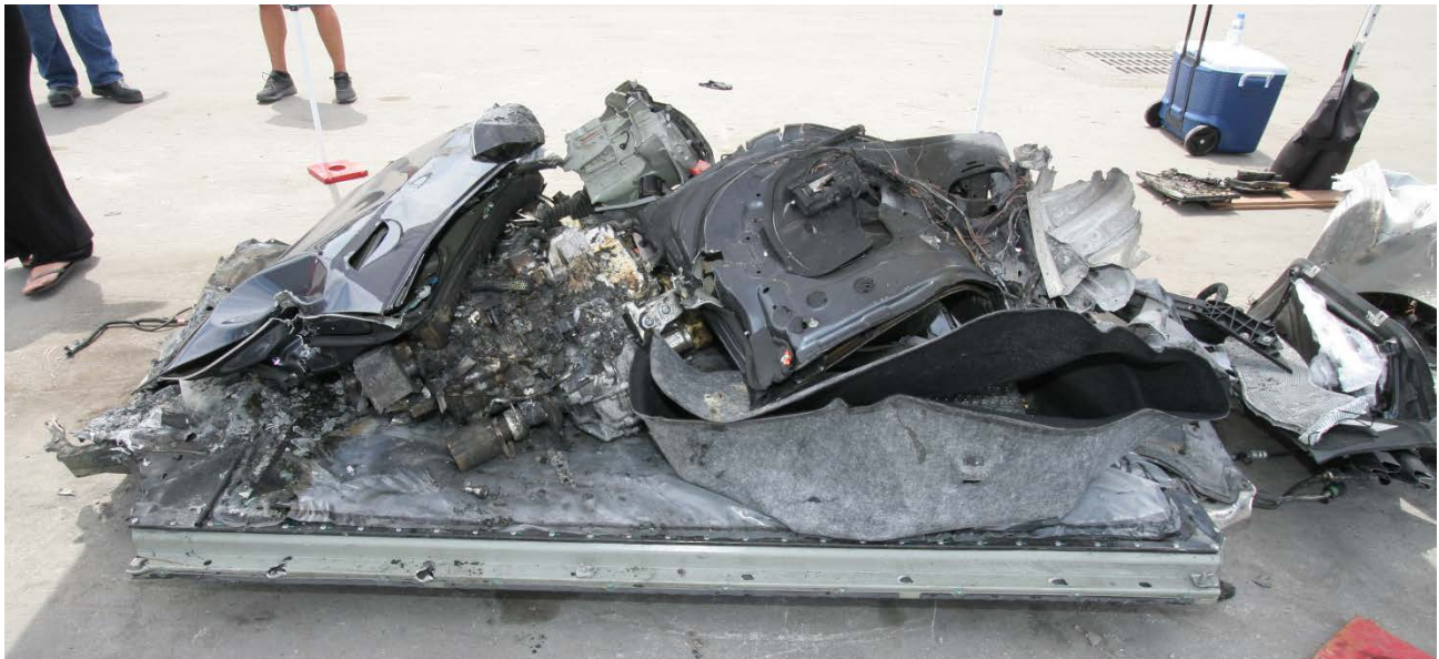
Figure 7: Battery pack with vehicle debris piled on top.
