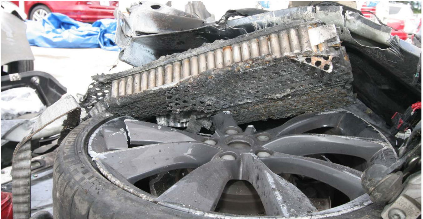
Figure 8: Fire damaged battery module.
