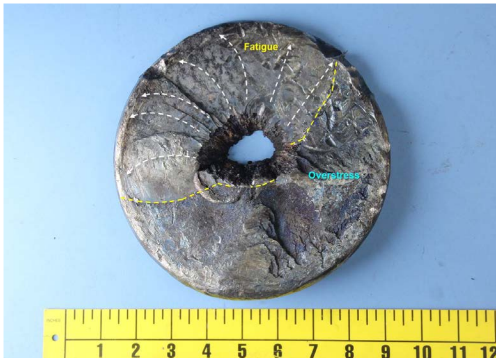
Figure 29. Fracture surface of the broken axle with fatigue and overstress areas labeled [Figure 8 of Reference 3].
