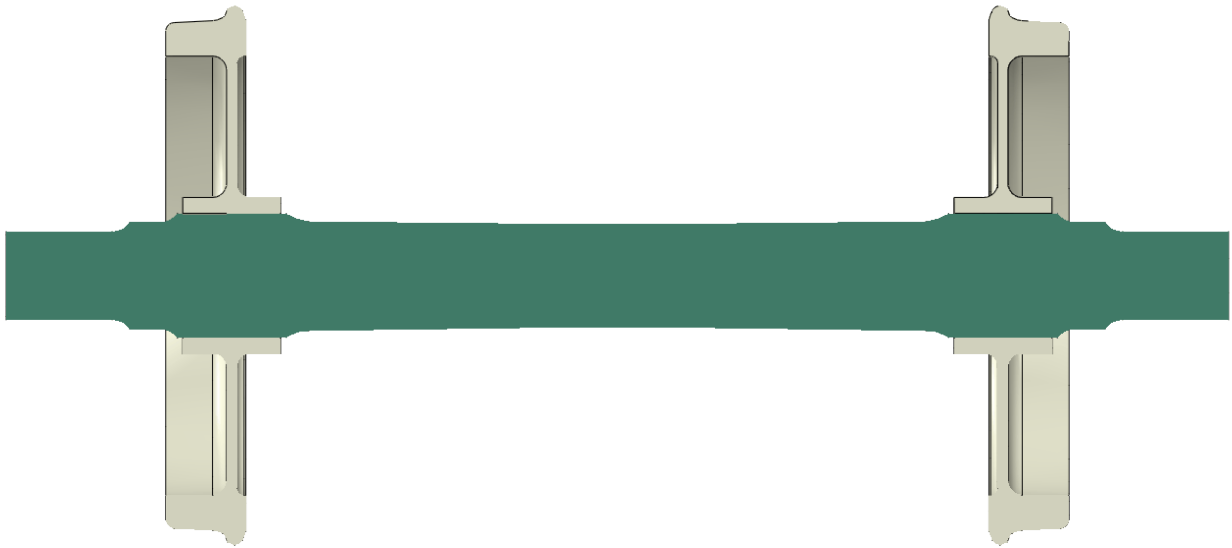
Figure 3. Created geometry of the wheelset, plan view.
