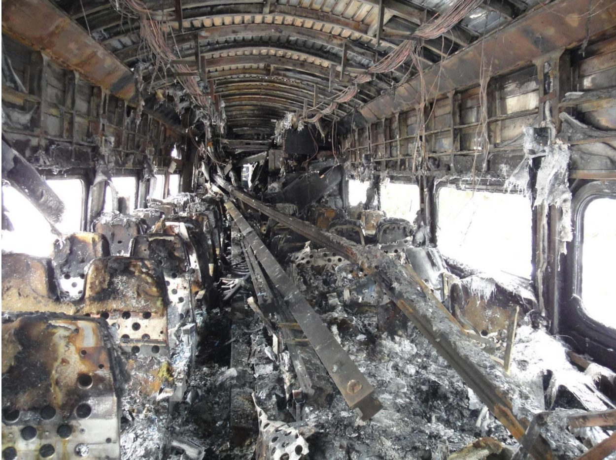
Figure 3. Postaccident photograph of the interior of the lead railcar.
