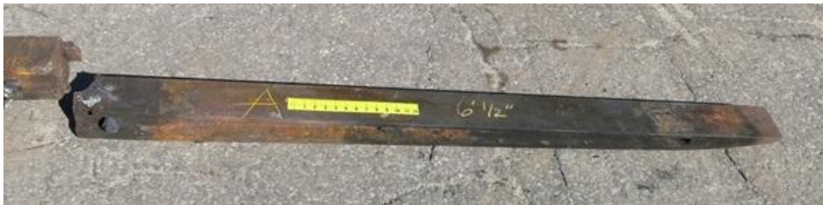
Figure 22. Third rail nose piece involved in this accident.
