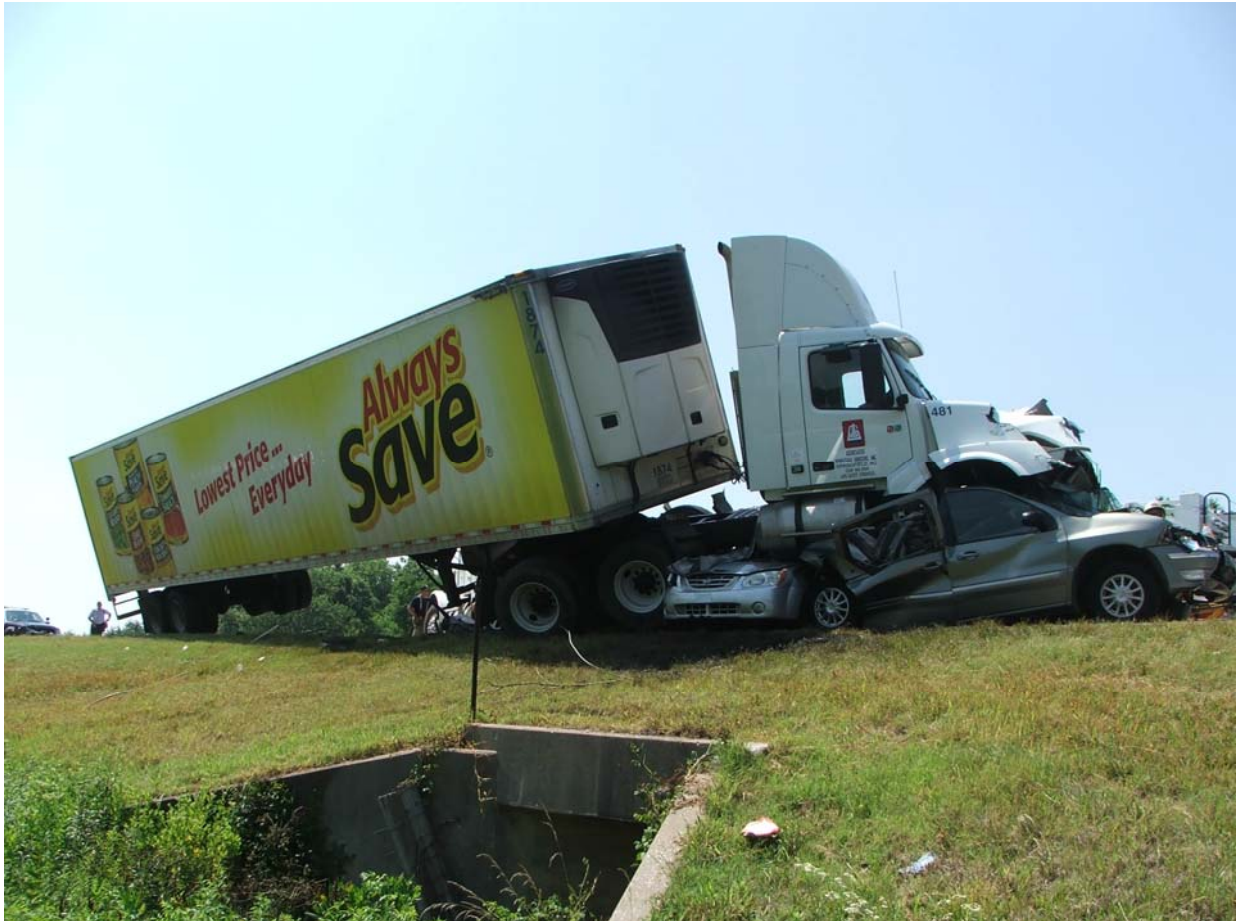
Figure 2. Postaccident photograph showing Volvo truck-tractor semitrailer override of passenger vehicles. [Photograph courtesy Oklahoma Highway Patrol]
