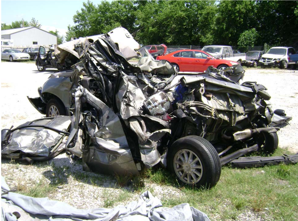
Figure B-4. Collision damage to 2000 Ford Windstar minivan.
