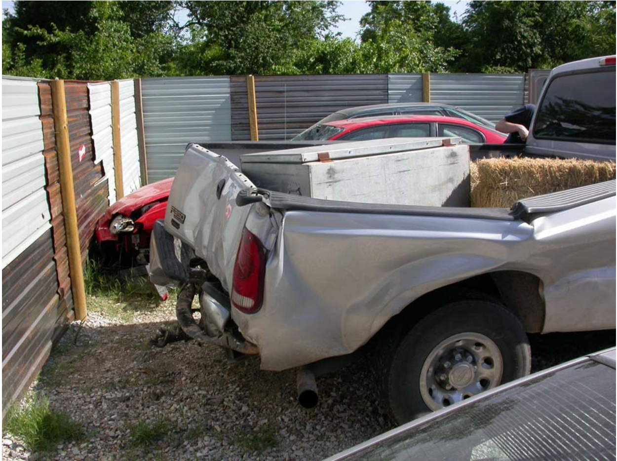
Figure B-6. Collision damage to 2004 Ford F350 pickup truck.
