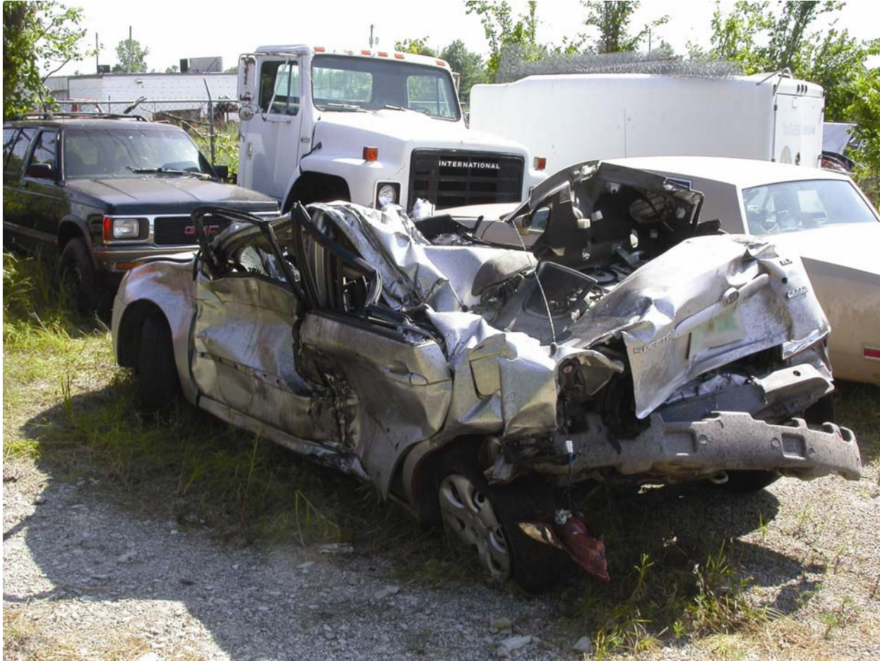
Figure B-3. Collision damage to 2004 Kia Spectra sedan.
