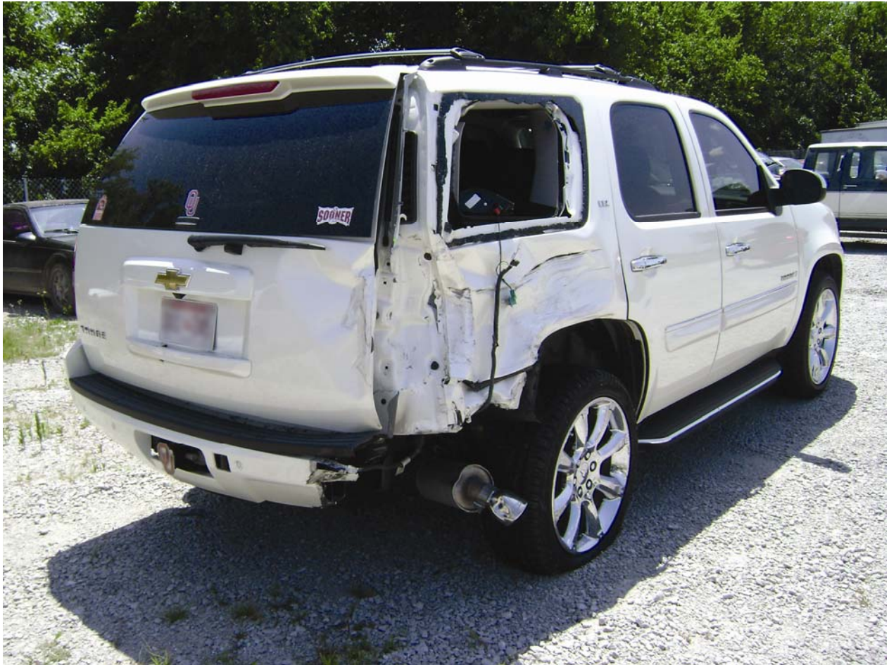
Figure B-7. Collision damage to 2008 Chevrolet Tahoe SUV.
