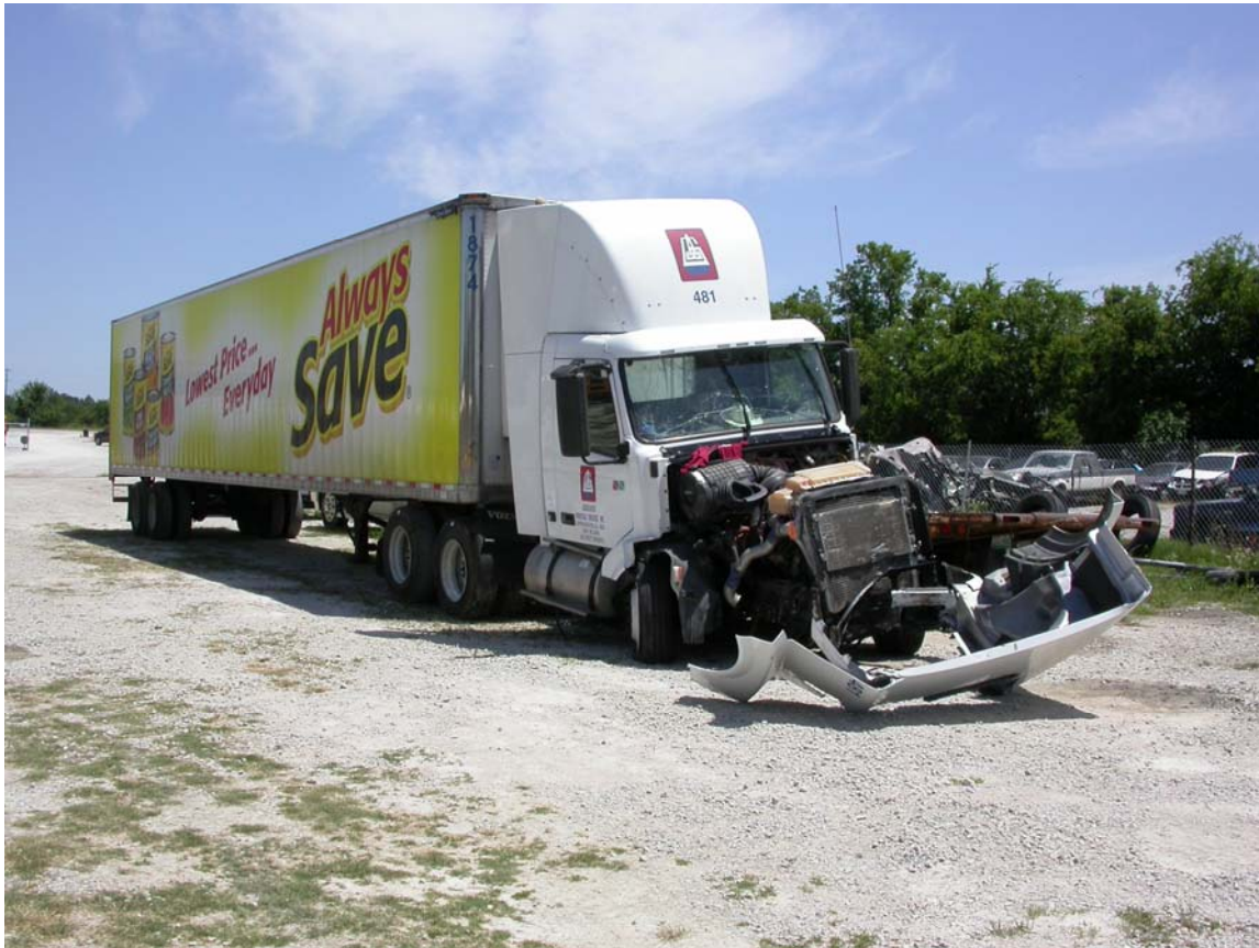
Figure 5. Collision damage to 2008 Volvo truck-tractor.
