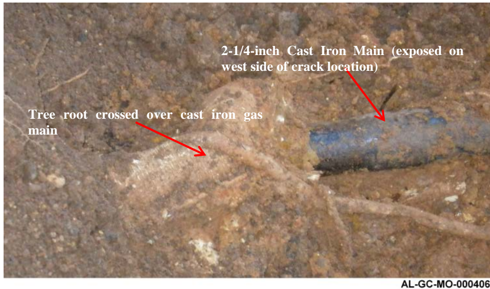
Figure 18: Root crossing over 2-1/4-inch cast iron main about 4 feet east of the crack location opposite Unit 80. Source: Alagasco
