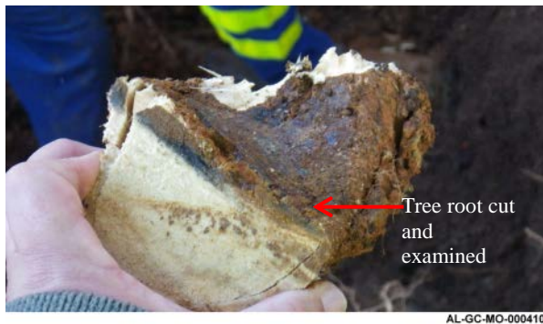
Figure 19: Tree root at the point of crossing 2-1/4-inch cast iron main opposite Unit 80. Source: Alagasco
