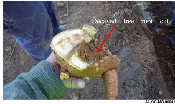
Figure 20: Surfaces of cut-out root where it rested on 2-1/4-inch cast iron main opposite Unit 80 (three photos shown). Source: Alagasco
