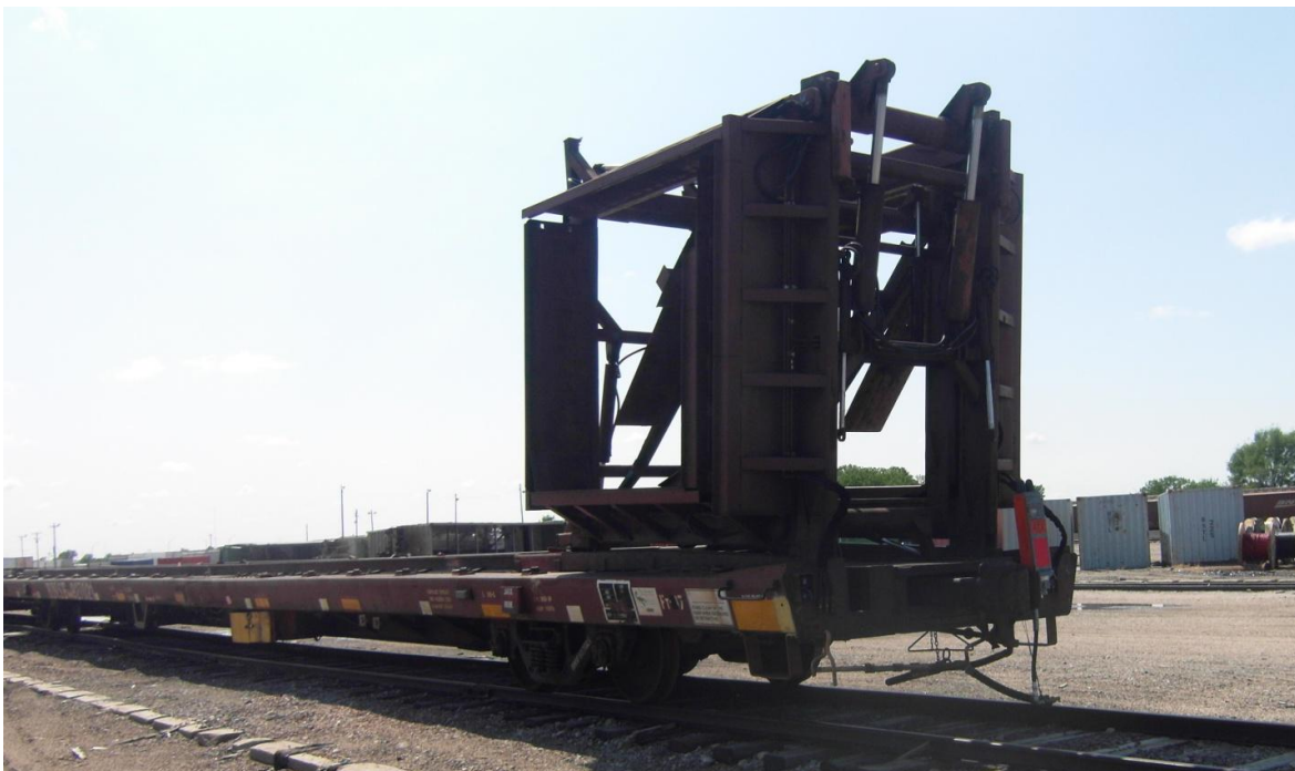
Figure 17. Exemplar scorpion-equipped flatcar.
