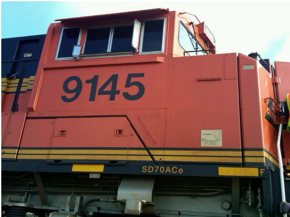
Figure 15. Exemplar EMD SD70ACe locomotive (same type as striking train locomotive) with modular cab.
