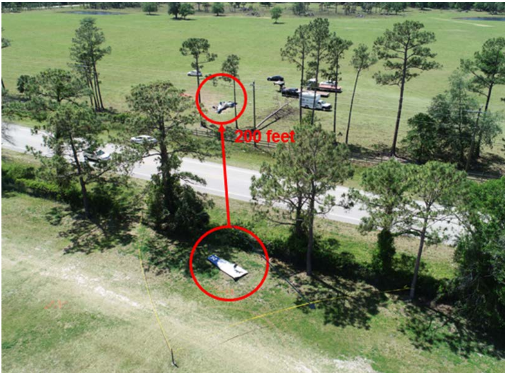
Figure 2. Photograph showing the separated left wing in foreground and main wreckage in background.
