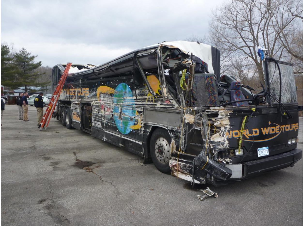
Figure 3 NTSB investigators examining motorcoach damage.
