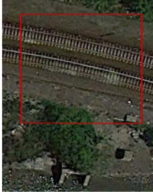
Figure 11: Satellite image from 2010 showing fouled ballast at POD
