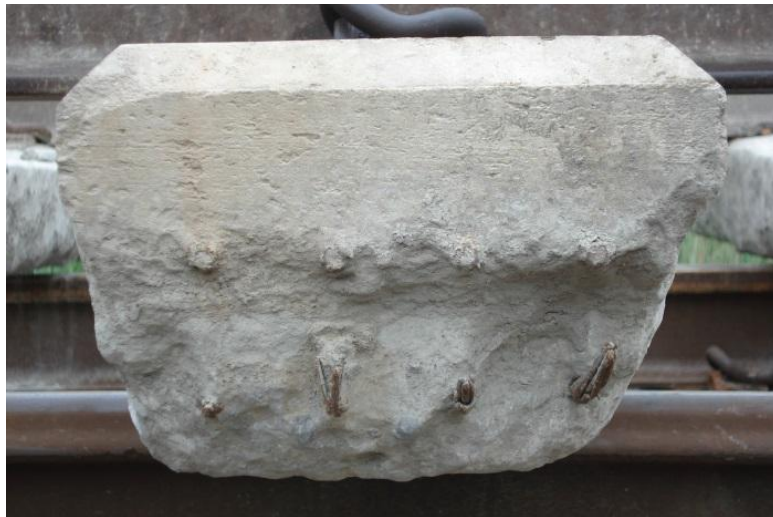
7 Figure 16: Tie from POD area with reduced cross-section and 8 exposed tension strands
