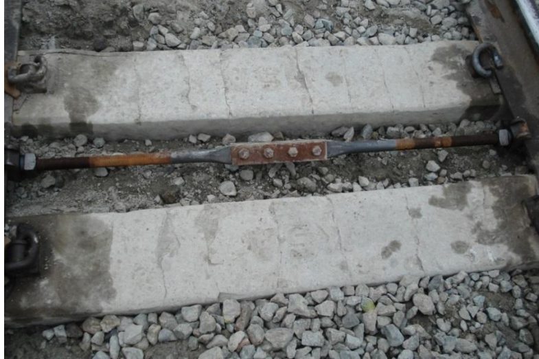
2 Figure 15: Cracks at centers of ties at POD (Note: gage rod was 3 installed after the derailment)
