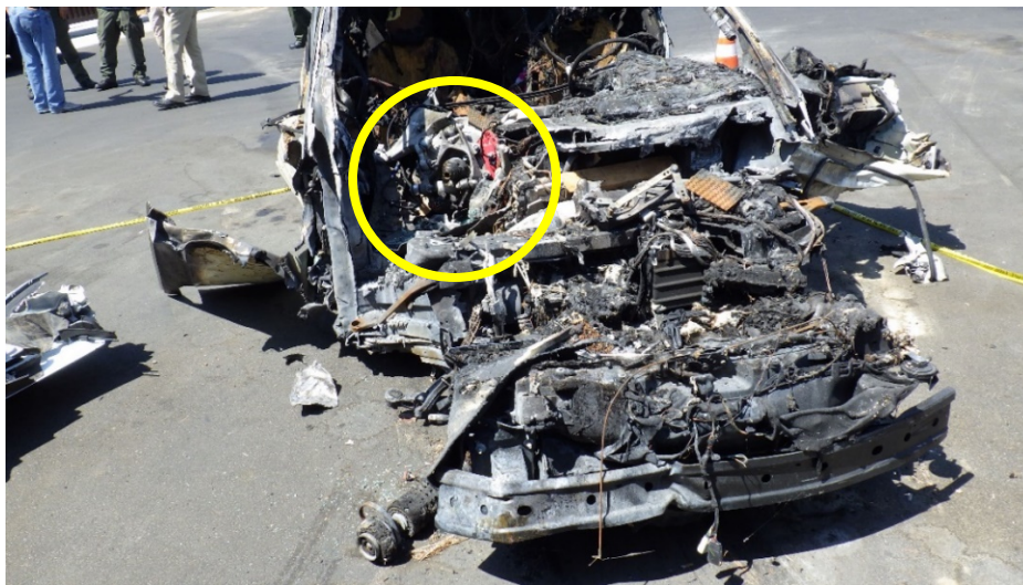
Figure 7: Front of Tesla with portions of right front wheel and other associated components circled in yellow
