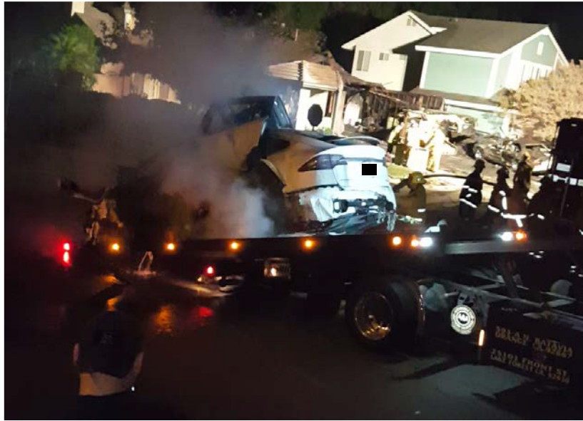
Figure 20: Tesla reignited on the flatbed towtruck. (source: OCFA)
