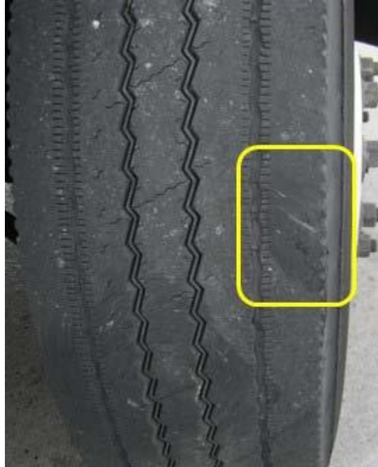
Figure 4. Abrasion on Right Front Tire of Truck Tractor (NTSB photograph)
