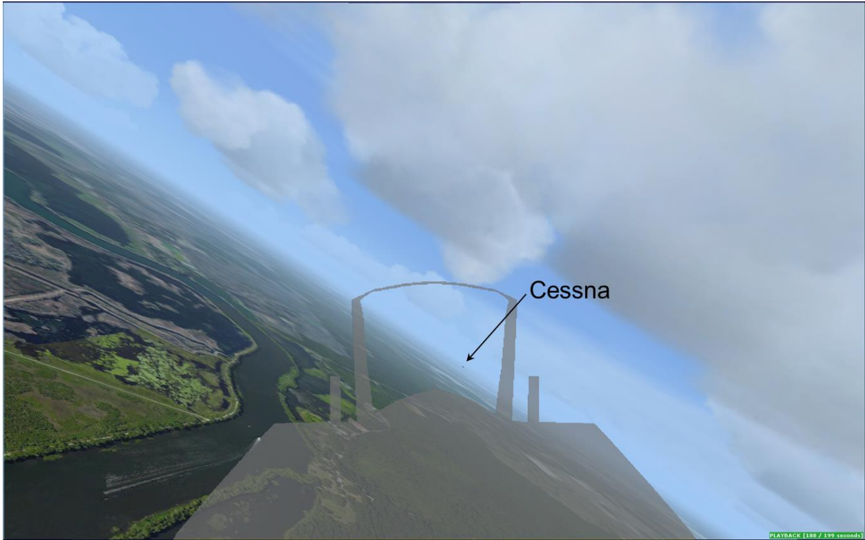
Figure 5a. Simulated cockpit visibility from the F-16 at 1100:49, when the airplanes were 0.6 nm apart.
