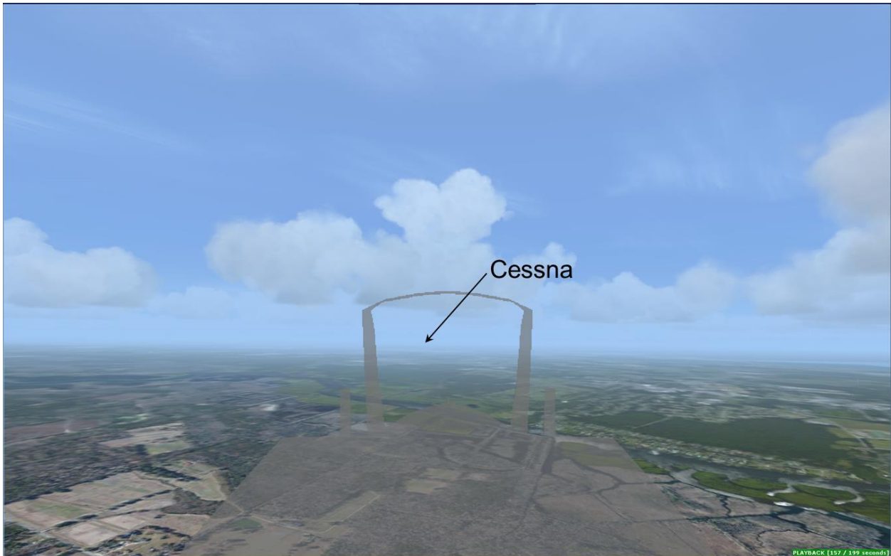
Figure 3a. Simulated cockpit visibility from the F-16 at 1100:18, when the airplanes were 3.1 nm apart. (Transparent shadow masks depict areas where visibility is obscured by airplane structure.)
