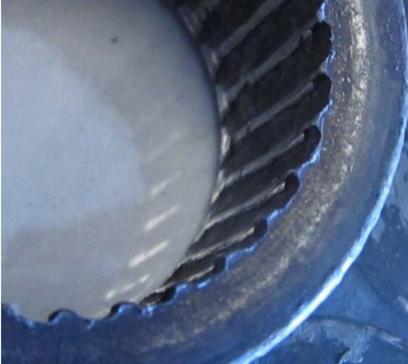
Photo 1 – Drive Disk Adapter - The thicknesses of the walls between the spline grooves on the drive disk adapter were reduced by more than 75% due to wear. The remaining thinned-edges of the groove walls were bent over due to rotation of the spline shaft within the drive disk adapter.
