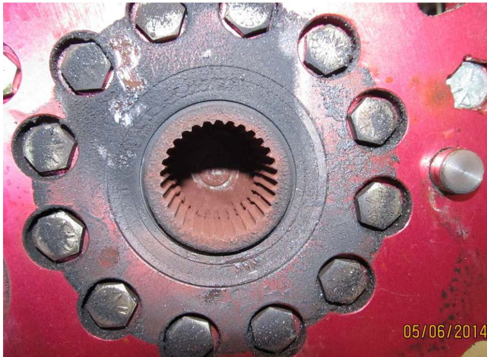
Photo 8 – The PSRU input spline groove walls are severely worn. There was about 1 teaspoon of red dust in the cavity. The presence of red dust is consistent with fretting wear.
