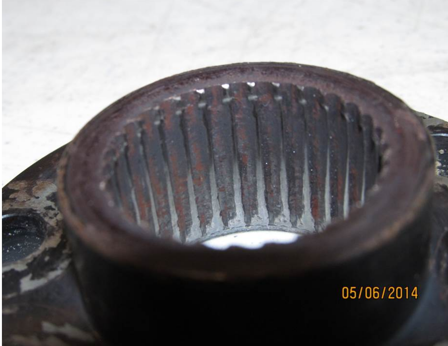
Photo 7 - Severe wear of the groove walls on the drive disk adapter.
