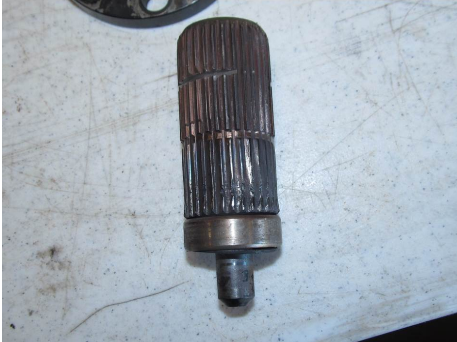
Photo 5 –There was direct mechanical damage and more than 75% wear of the spline teeth on the engine end of the spline shaft. The tips of the spline teeth were rolled over. The cuts on the PSRU-end of the drive shaft were made to facilitate the use of a puller. There is more than 25% wear of the spline teeth on the PSRU end of the spline shaft.
