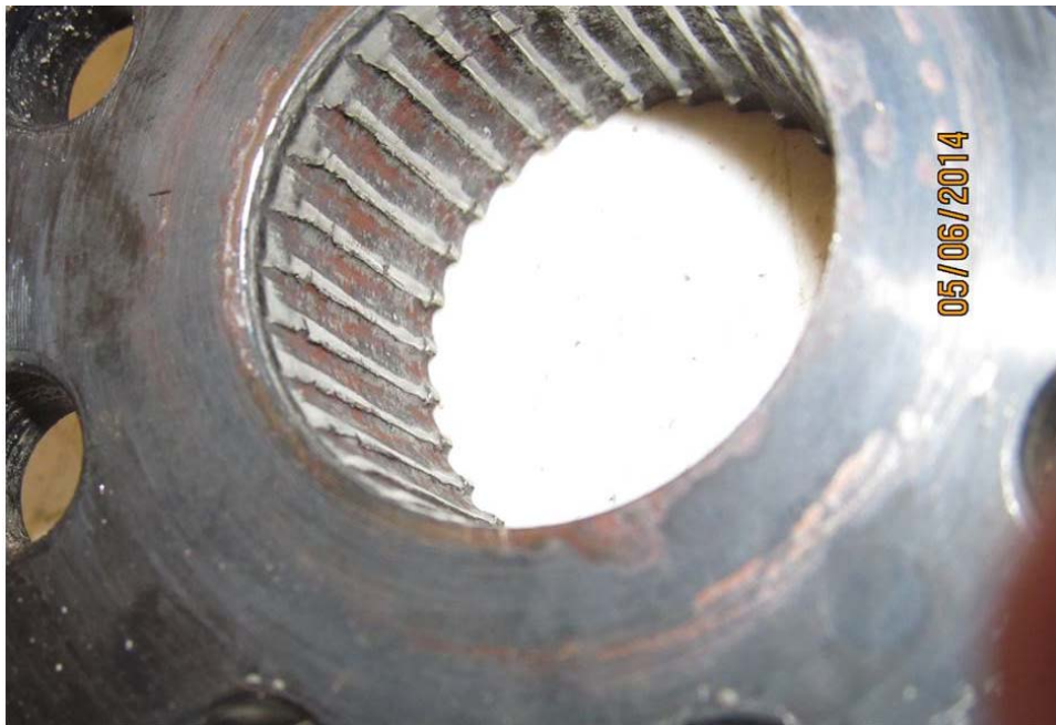
Photo 6 –There was over 75% wear of the walls on the drive disk adapter. The tips of the walls were bent over.
