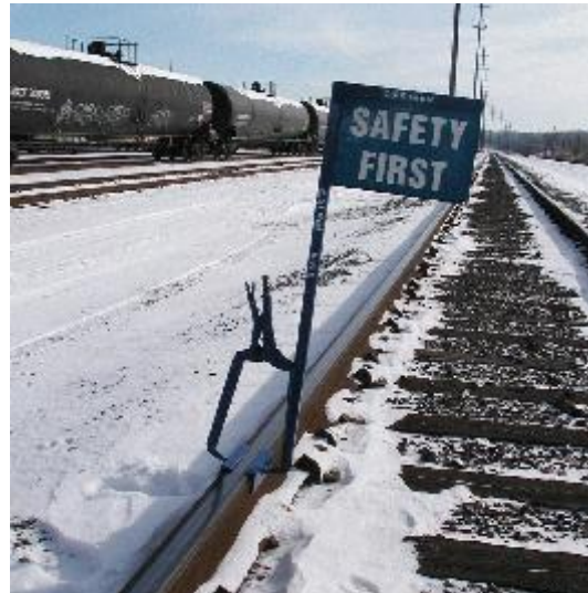
Blue Signal Sign attached to snow covered track in a trainyard
