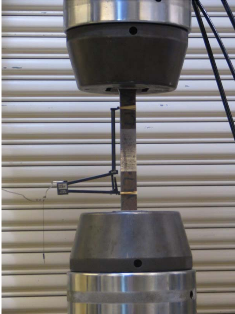
Figure 3 Gusset plate tension test using MTS self-aligning grips and extensometer with an 8 in. gage length.
