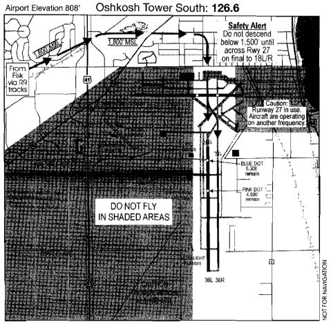
The RWY 18R relocated threshold is abeam the air traffic control tower and is marked by Runway End Identification Lights and orange lines.
