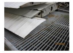
The right wing tip also sustained damage but it was not as severe as the left wing. The wing tip was removed after the accident. There were no indications of torsion on the right wing root.
