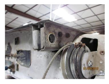
FAA Inspector Josh Brown found a cracked and deformed rear spar in the left wing. The cracked and deformed spar, by FAA standards, classified this as an accident.
