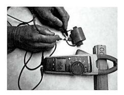
The upper limit of the primary coil windings were .6 Ohms higher than the limit of 1.2 Ohms that is published in the maintenance manual. There is no published resistance reading for a "hot" coil that we could compare it to.
