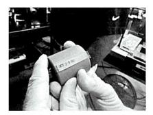
The coil was then placed in a calibrated oven at 201 degrees for 2 hours.
