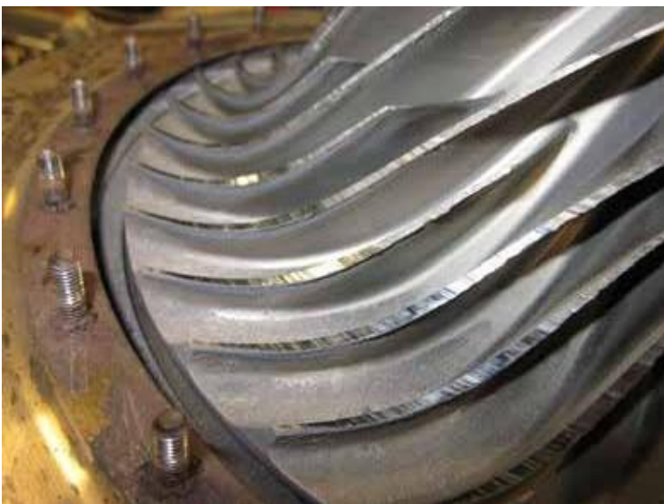
Figure 12, Impeller, rub marks shown
