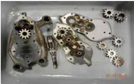
Figure 21, Oil Pump, disassembled
