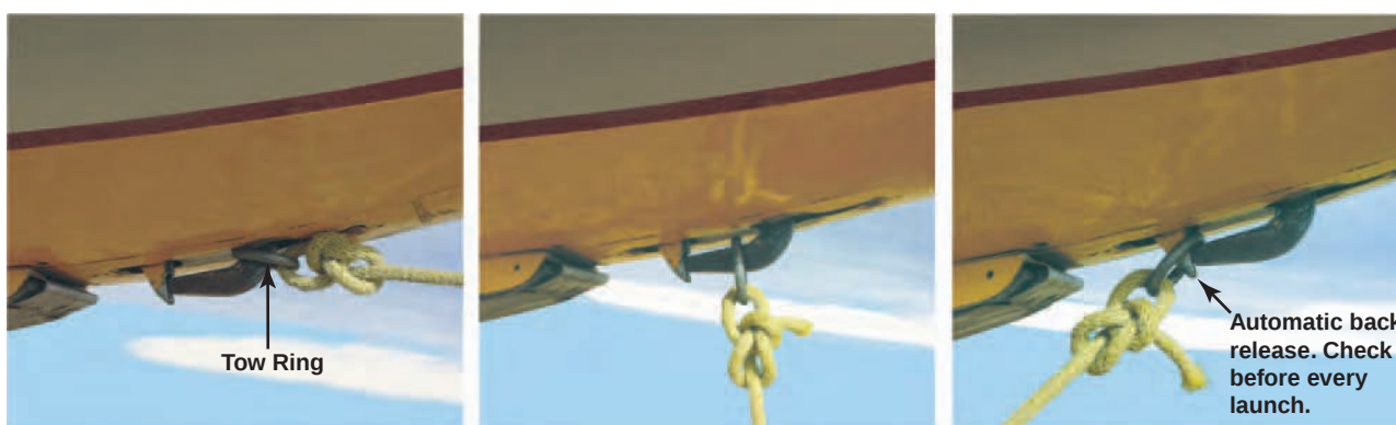
Figure 7-13. Testing the towhook.
