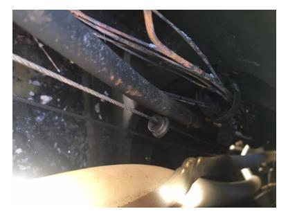
In this area were two clamps, wiring can be seen passing thru one clamp, other clamp was missed by wiring and pinched against the rib. This is also the area where the paint was bubbled and burned on top of the wing.
