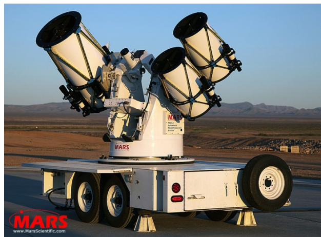
Figure 1: An example of a 3 camera MARS system mounted on a trailer based tracking mount. (photo: MARS Scientific)
