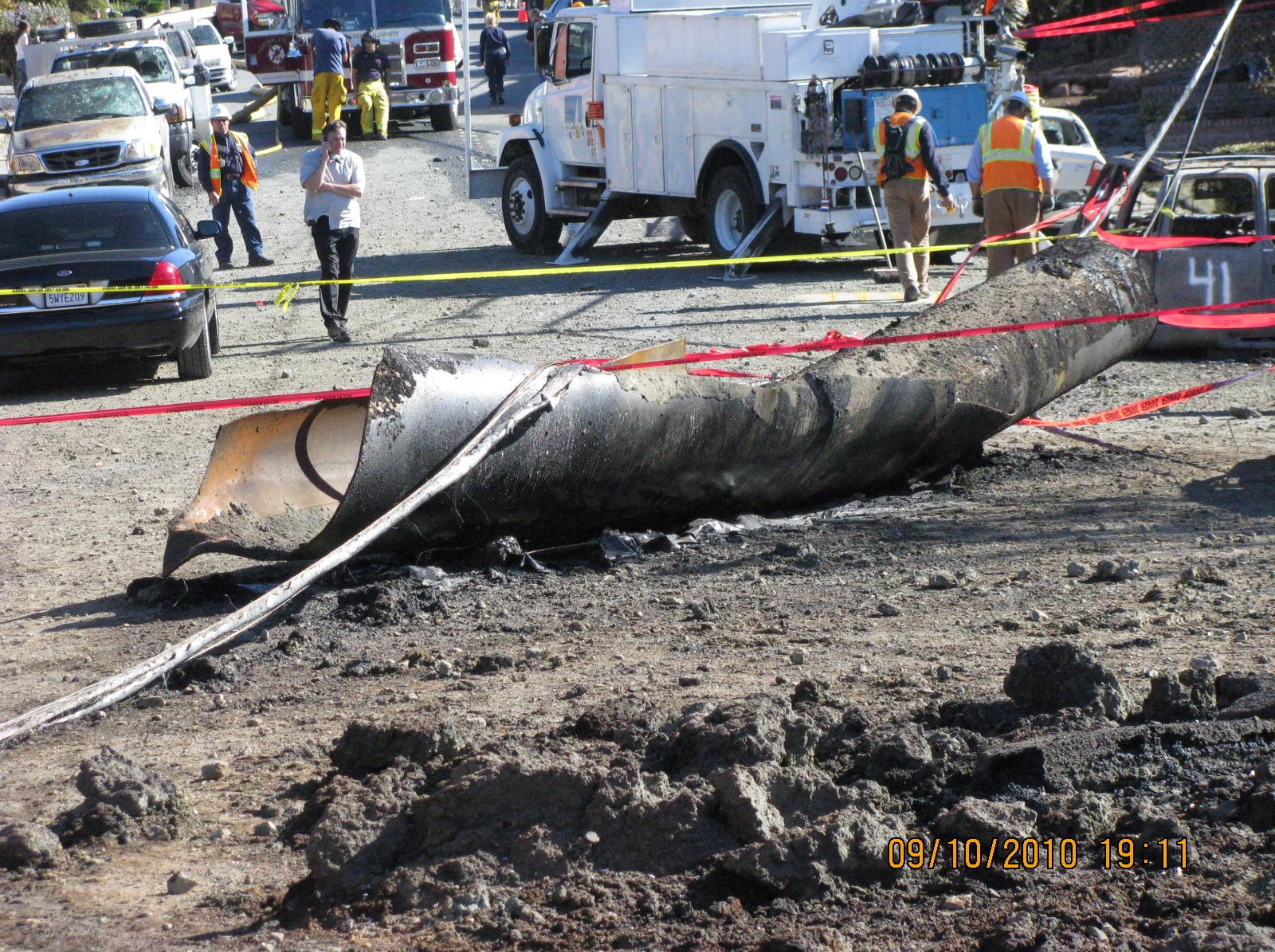
Exhibit 2CX: Segment of Ruptured Pipeline Resting in Glenview Avenue, 10 Sept 2010 IMG_0098 NTSB (Downs)
