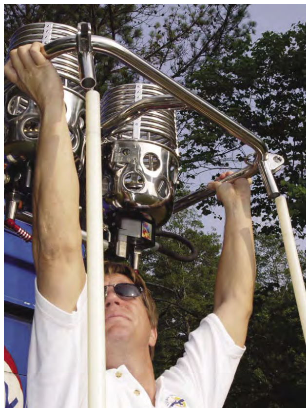
Figure 6-9. Burner installation on a Lindstrand.
