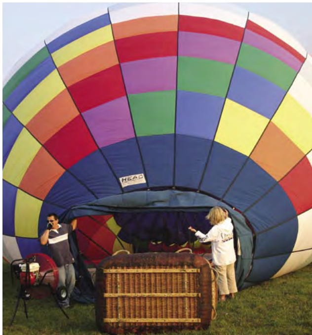
Figure 2-12. Balloon inflation using a typical inflation fan.
