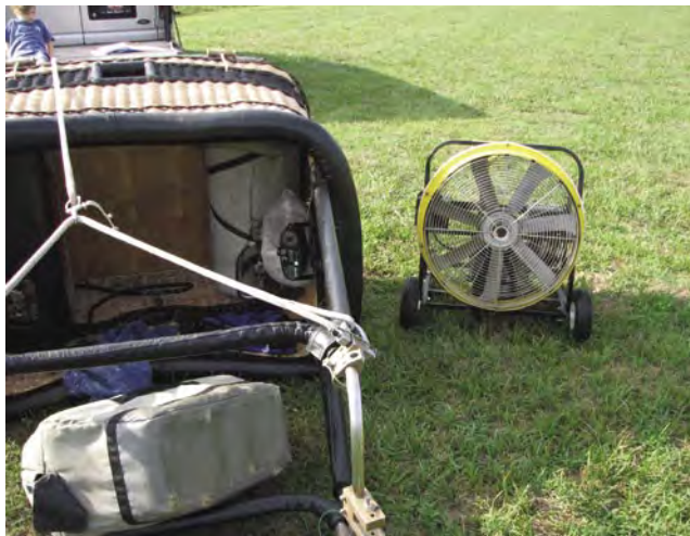
Figure 6-13. Placement of the inflation fan.
