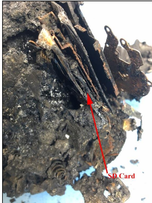
Figure 35. The device shown with an arrow indicating the SD card's position.
