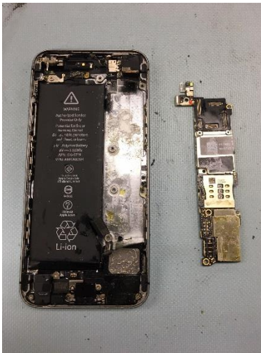
Figure 21. The device opened with the main board removed.
