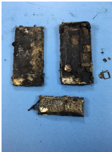
Figure 11. The iPhone after being opened. The internal memory board was thermally destroyed.
