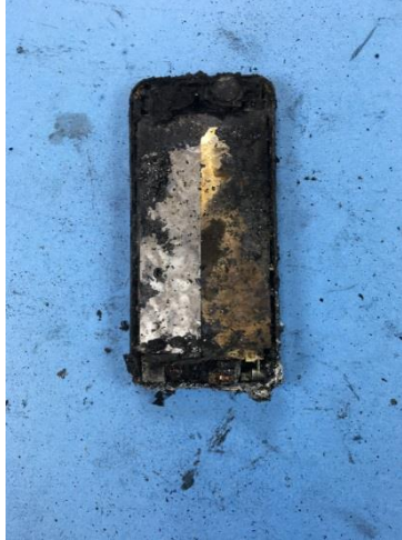
Figure 14. The iPhone after being opened. The internal memory board was thermally destroyed.
