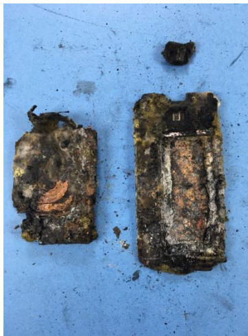
Figure 17. The device's internal components after being opened.
