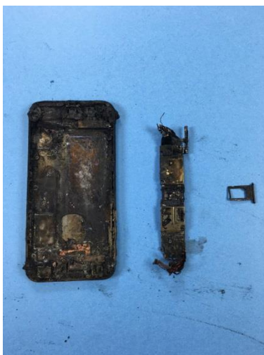
Figure 6. Photo with memory board and SIM chassis removed.
