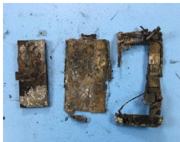
Figure 13. The iPhone after being opened. The internal memory board was thermally destroyed.
