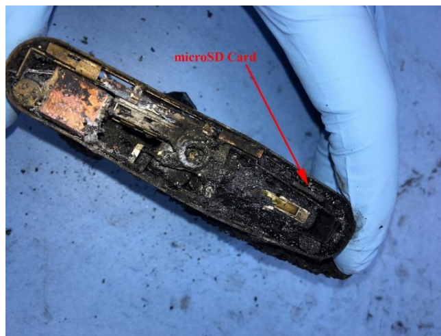
Figure 32. The device shown with an arrow indicating the microSD card's position.
