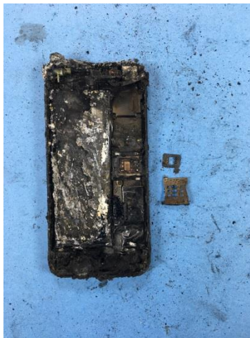
Figure 15. The iPhone after being opened. The internal memory board was thermally destroyed.
