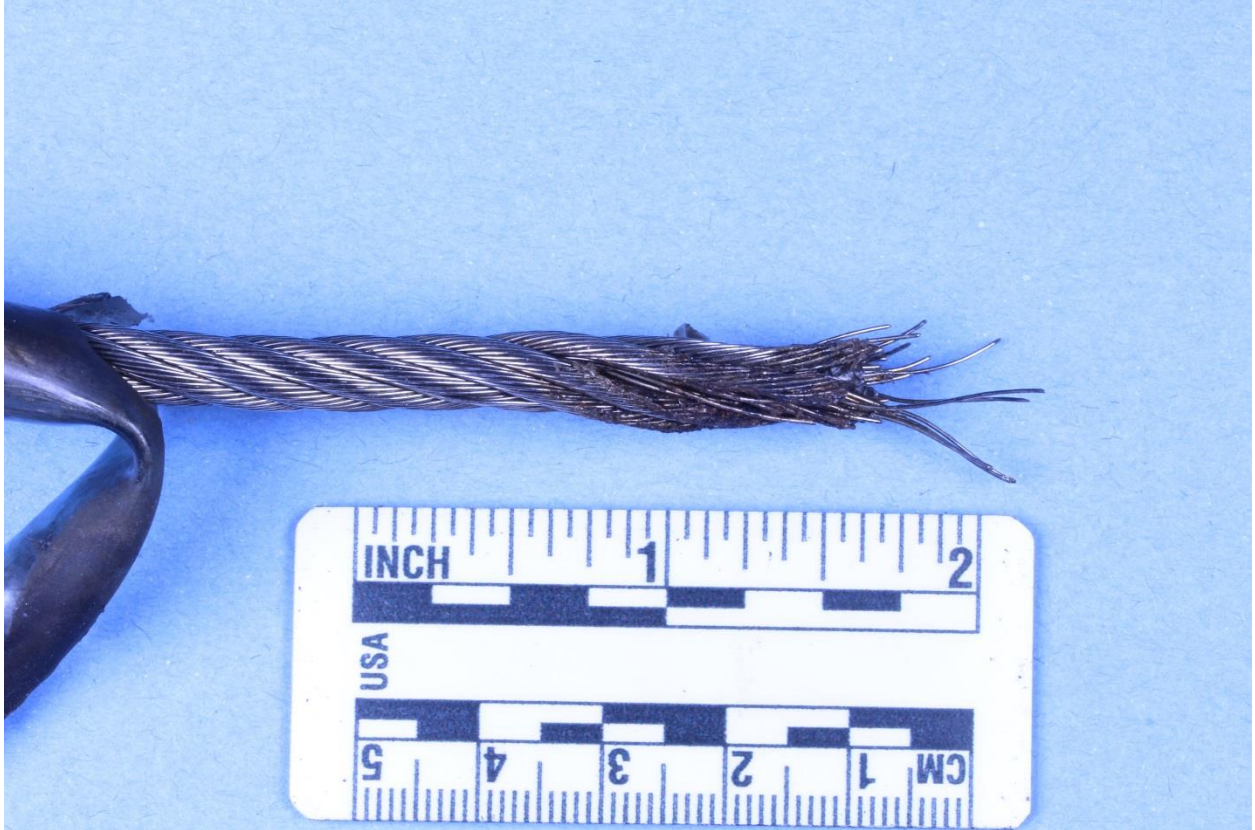
Figure 2: Severed cable end exhibiting strand fusing (Burner Support Frame 1)
