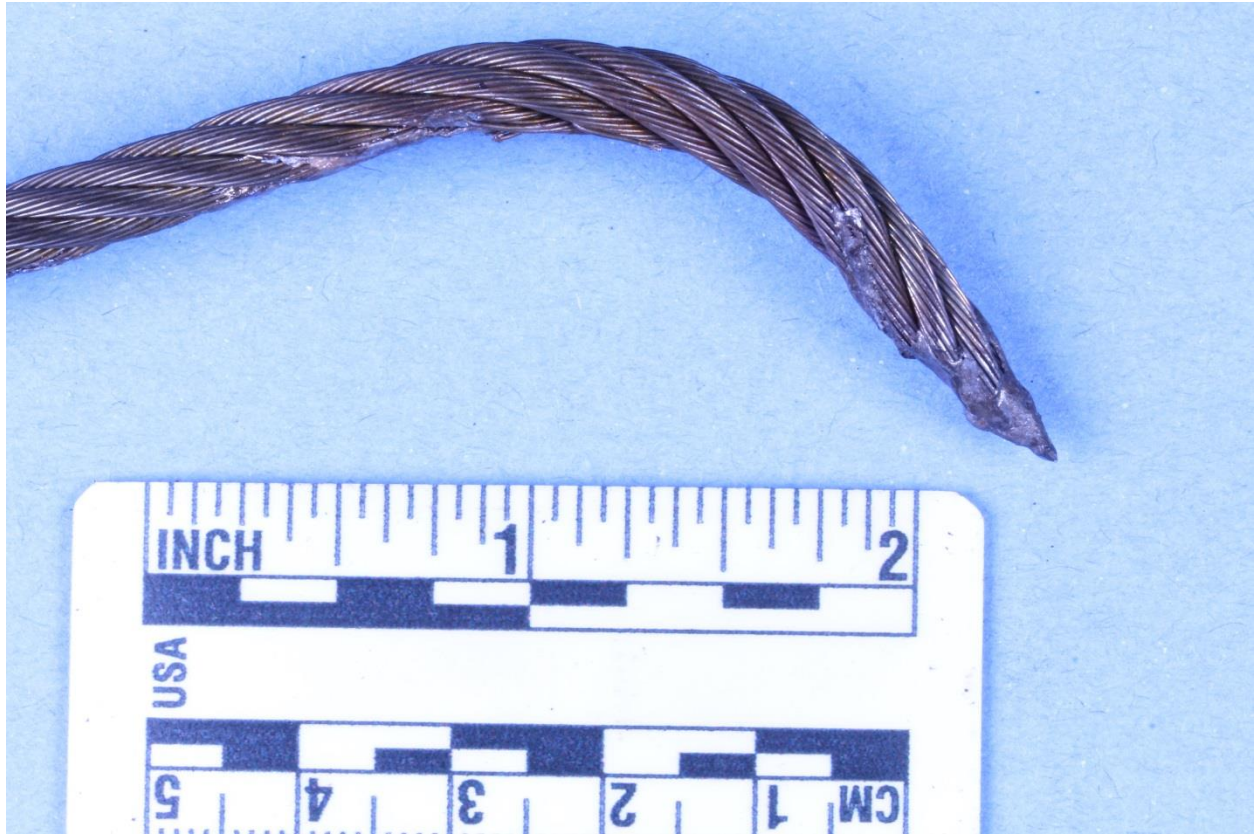
Figure 7: Basket cable exhibiting strand fusing (Burner Support Frame 2)
