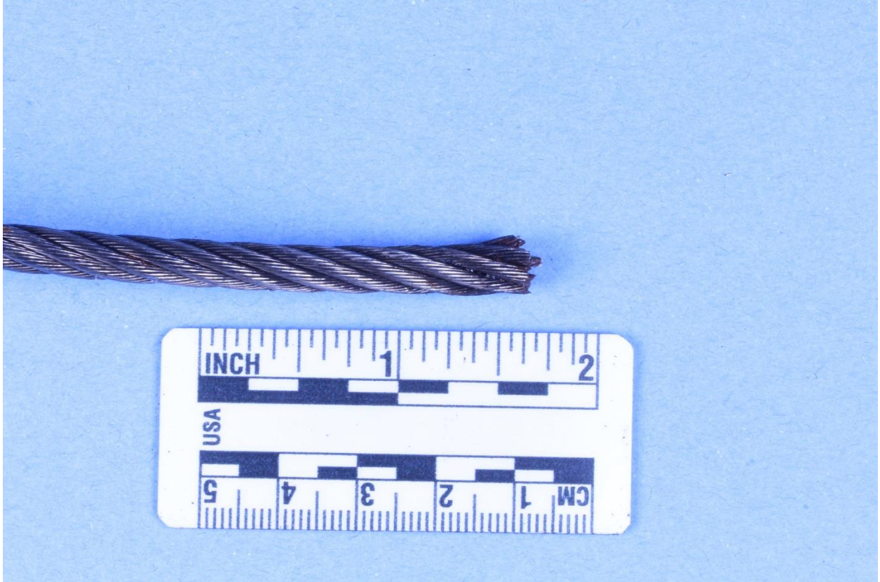
Figure 12: Basket cable exhibiting strand fusing (Burner Support Frame 4)
