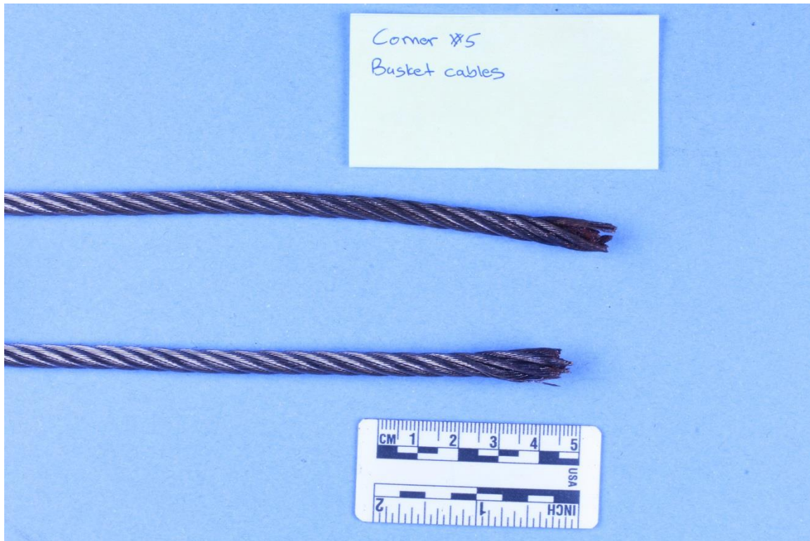
Figure 15: Basket cables exhibiting strand fusing (Burner Support Frame 5)
