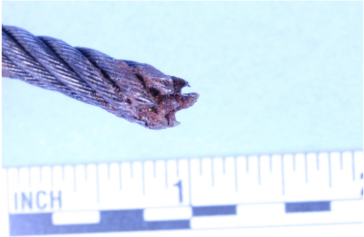
Figure 8: Basket cable exhibiting strand fusing (Burner Support Frame 3)
