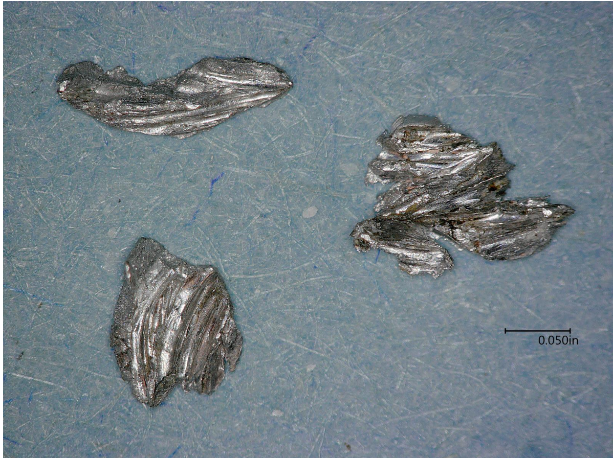
Figure 14: shavings of aluminum recovered from cable exterior (Burner Support Frame 4)
