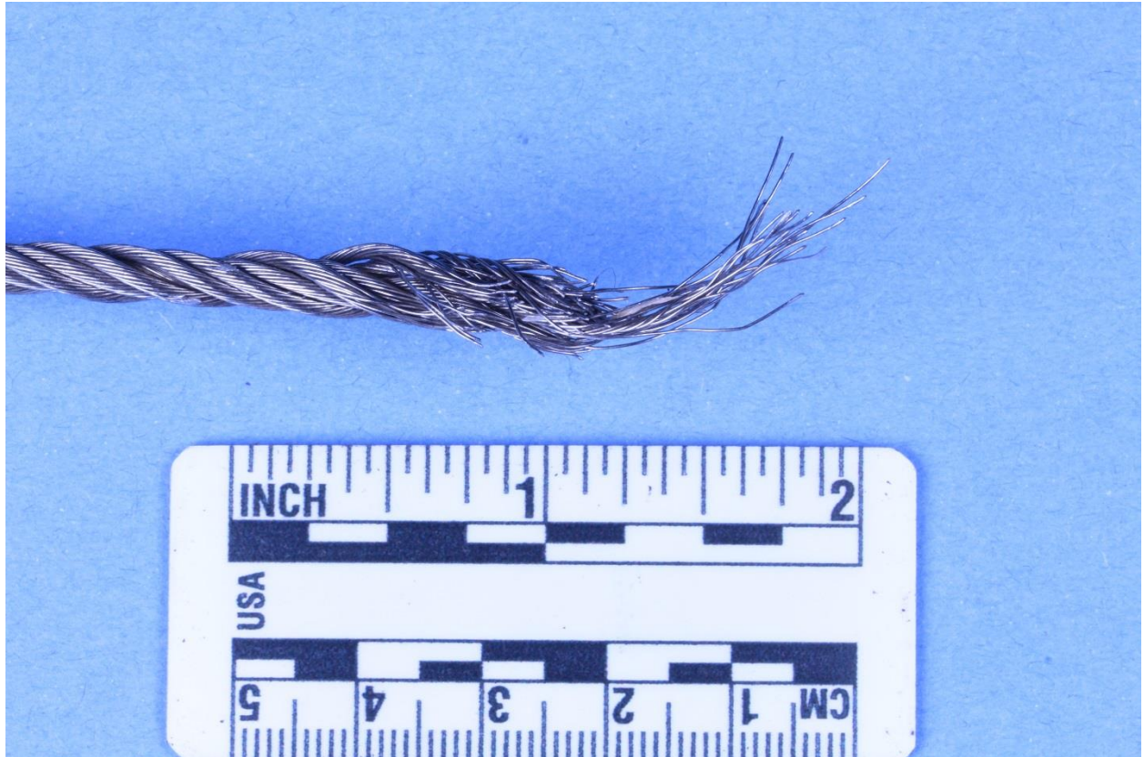
Figure 5: Load cable exhibiting overload failure (Burner Support Frame 1)
