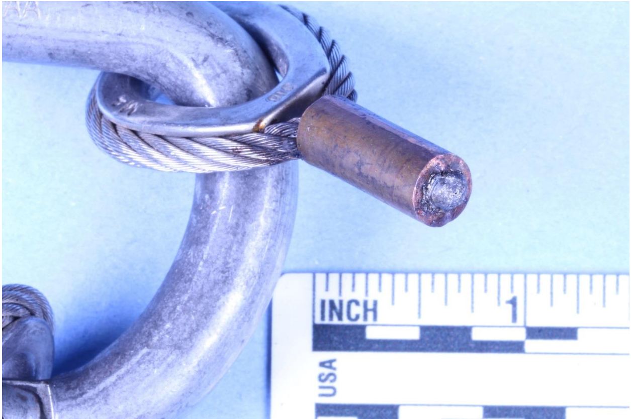
Figure 9: Load cable exhibiting strand fusing at the eyelet (Burner Support Frame 3)
