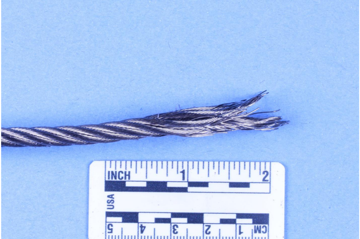
Figure 11: Basket cable exhibiting overload (Burner Support Frame 4)
