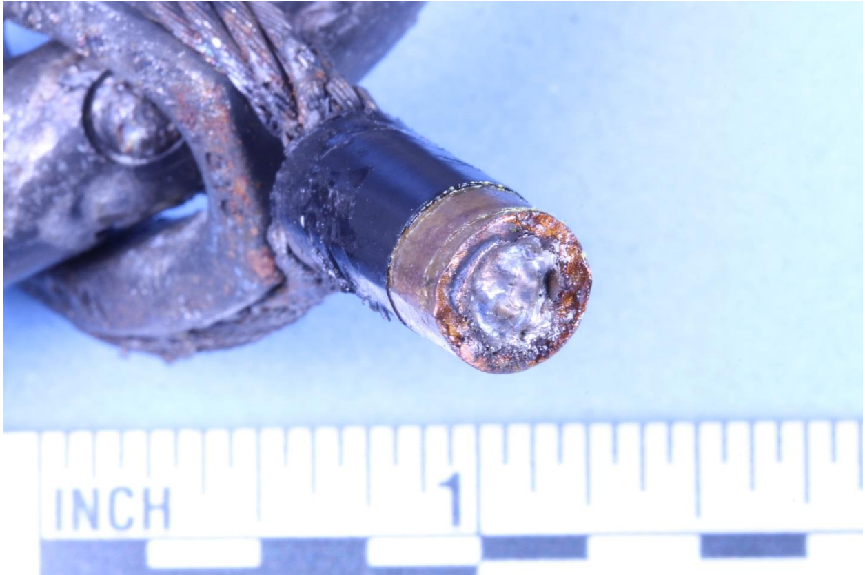
Figure 4: Load cable fused and separated at eyelet (Burner Support Frame 1)
