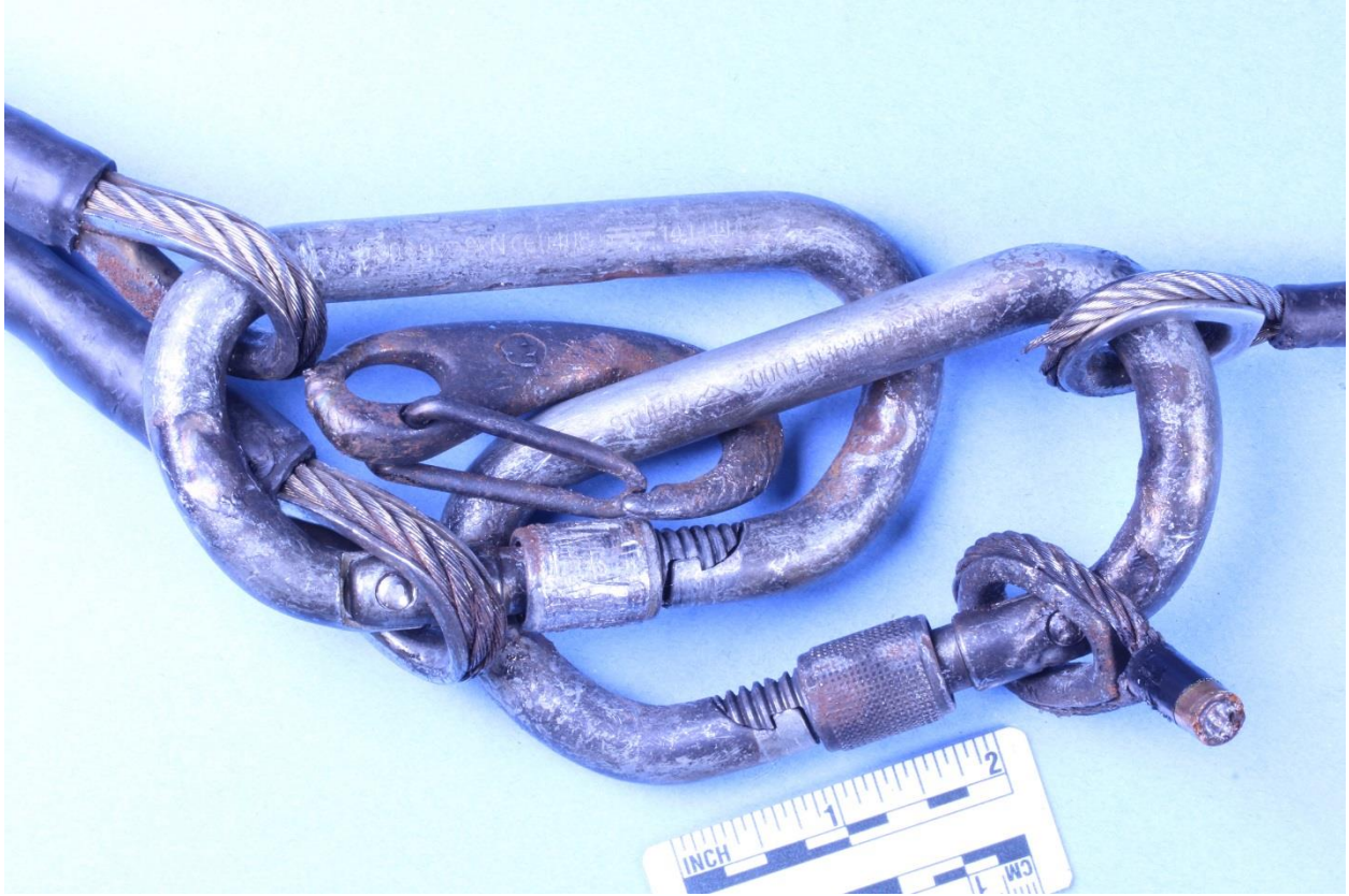
Figure 3: Carabiners with electrical arcing damage (Burner Support Frame 1)
