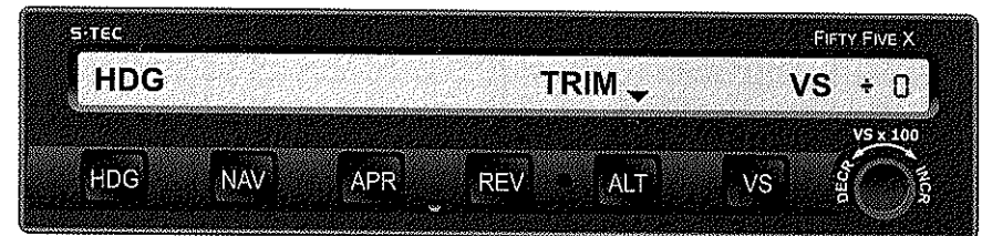
b. HDG and VS Modes Engaged, 0 FPM, TRIM DN in Progress
