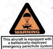
located on the both sides of fuselage between canopy and rear window
