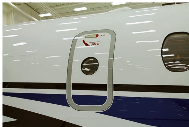
Figure 1-8. Emergency Exit (Exterior)
