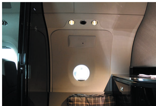
Figure 1-9. Emergency Exit (Interior)
