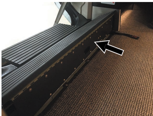
Figure 1-7. Water Barrier (Deployed)
