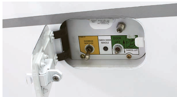
Figure 1-5. Exterior Door Control Panel
