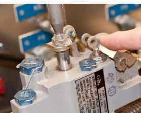
Input lever shown stuck in fully deployed position and stuck in mid position:
