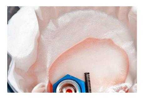
A little chip came out with fluid when medium blue plug was pulled (check valve).
