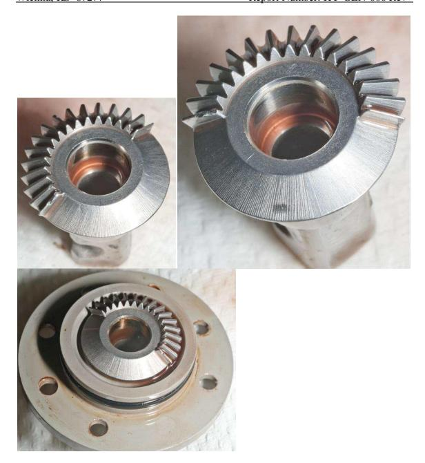
No visible damage to spool control summing gear or valve assembly.
