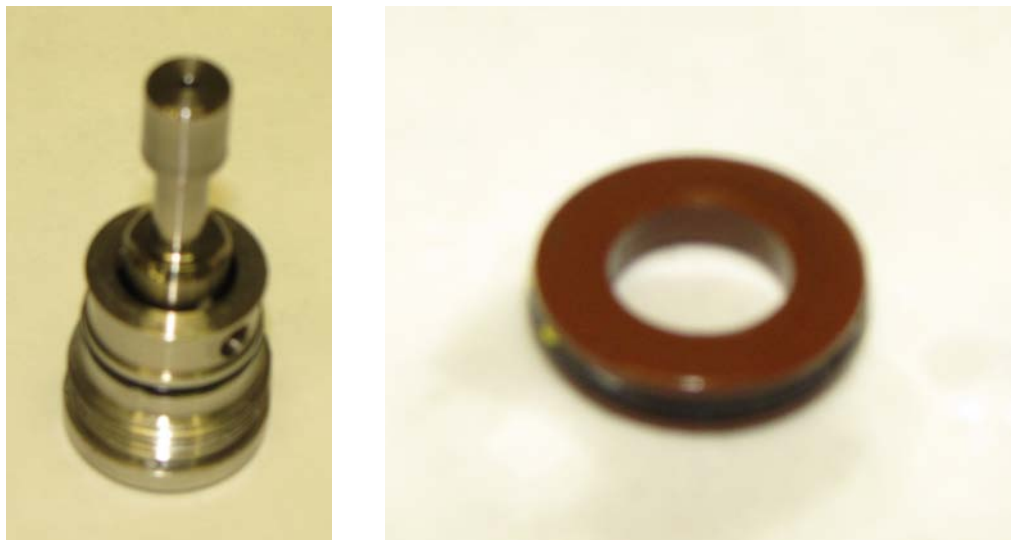
Figure 7. PV101 Poppet, Retainer and Seat.
