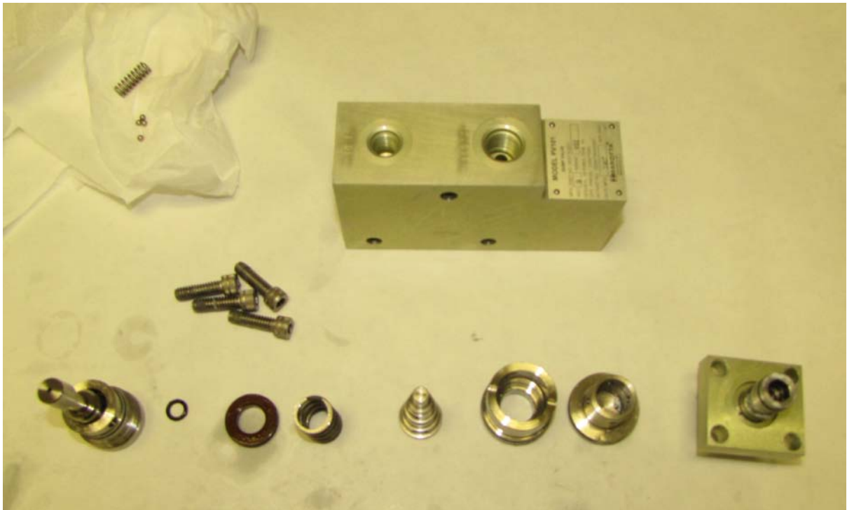
Figure 6. PV101 S/N481 completely disassembled.
