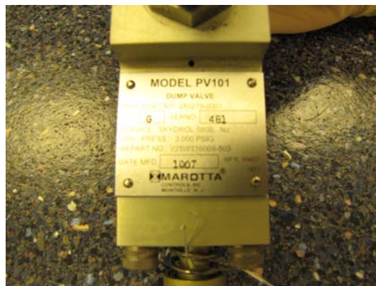
Figure 2. PV101 identification nameplate.
