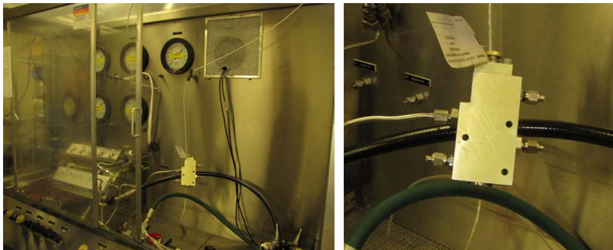
Figure 4. Marotta Skydrol LD-4 test stand with PV101 installed.
