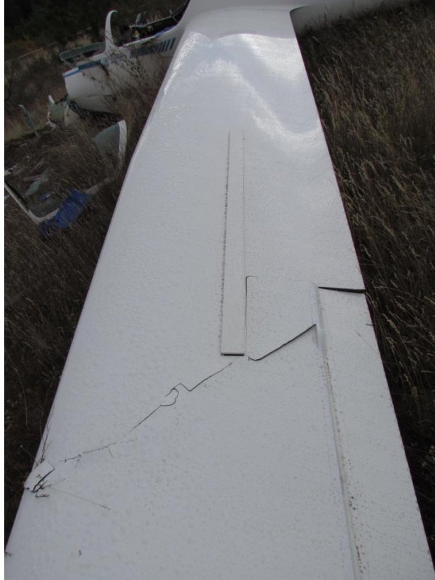
Figure 6: Left Wing Mid-span Chordwise Cracking
