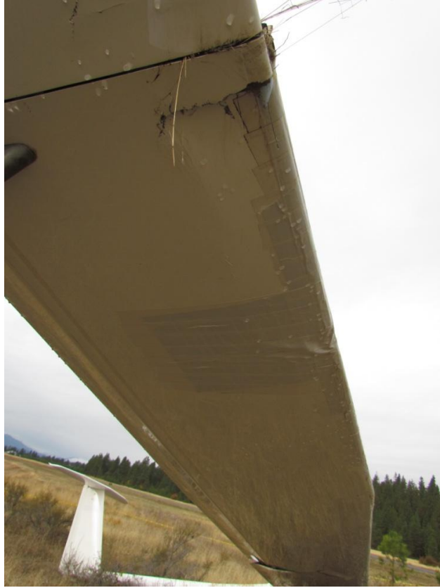
Figure 8: Bottom of Outboard Right Wing Repair
