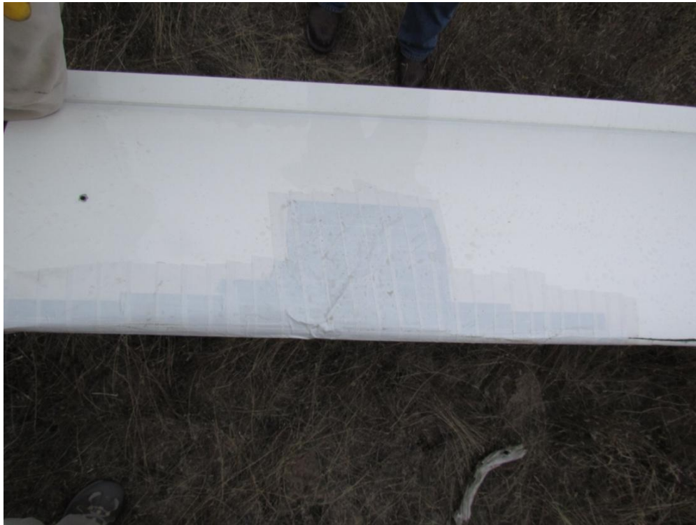
Figure 9: Top of Outboard Right Wing Repair
