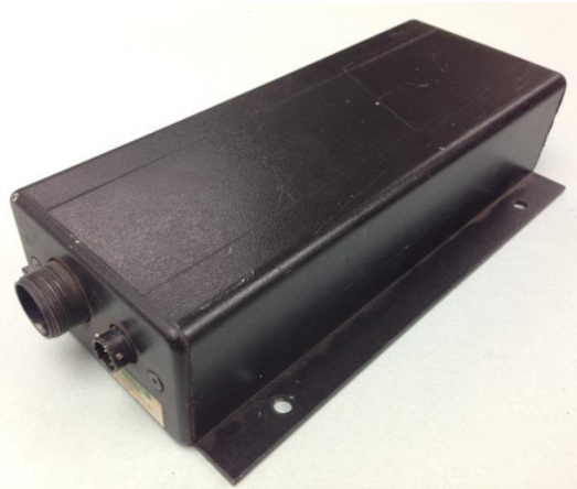
Figure 2. Siemens/Quantum Q1027 recorder from DPU locomotive CSX 7921.
