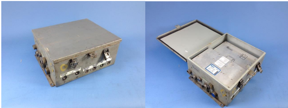
Figure 2. Siemens/Quantum Q1027 recorder from DPU locomotive CSX 7921.
