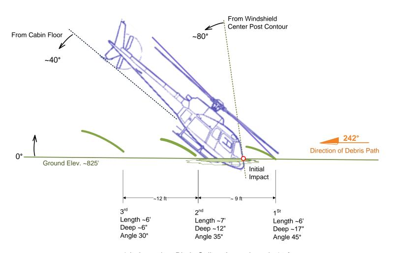
3 Independent Blade Strikes Approximately 15 ft to the Right of Wreckage Path (Left Side of aircraft)
