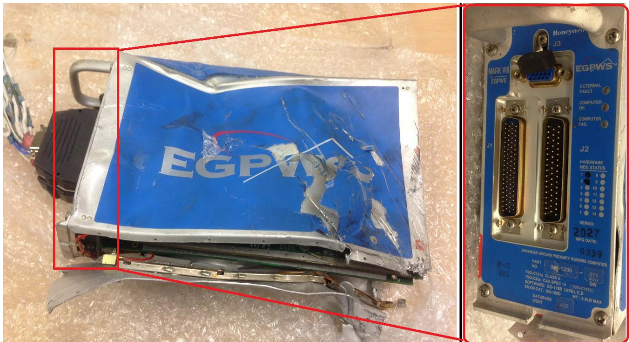
Figure 1. Damaged exterior of EGPWS.
