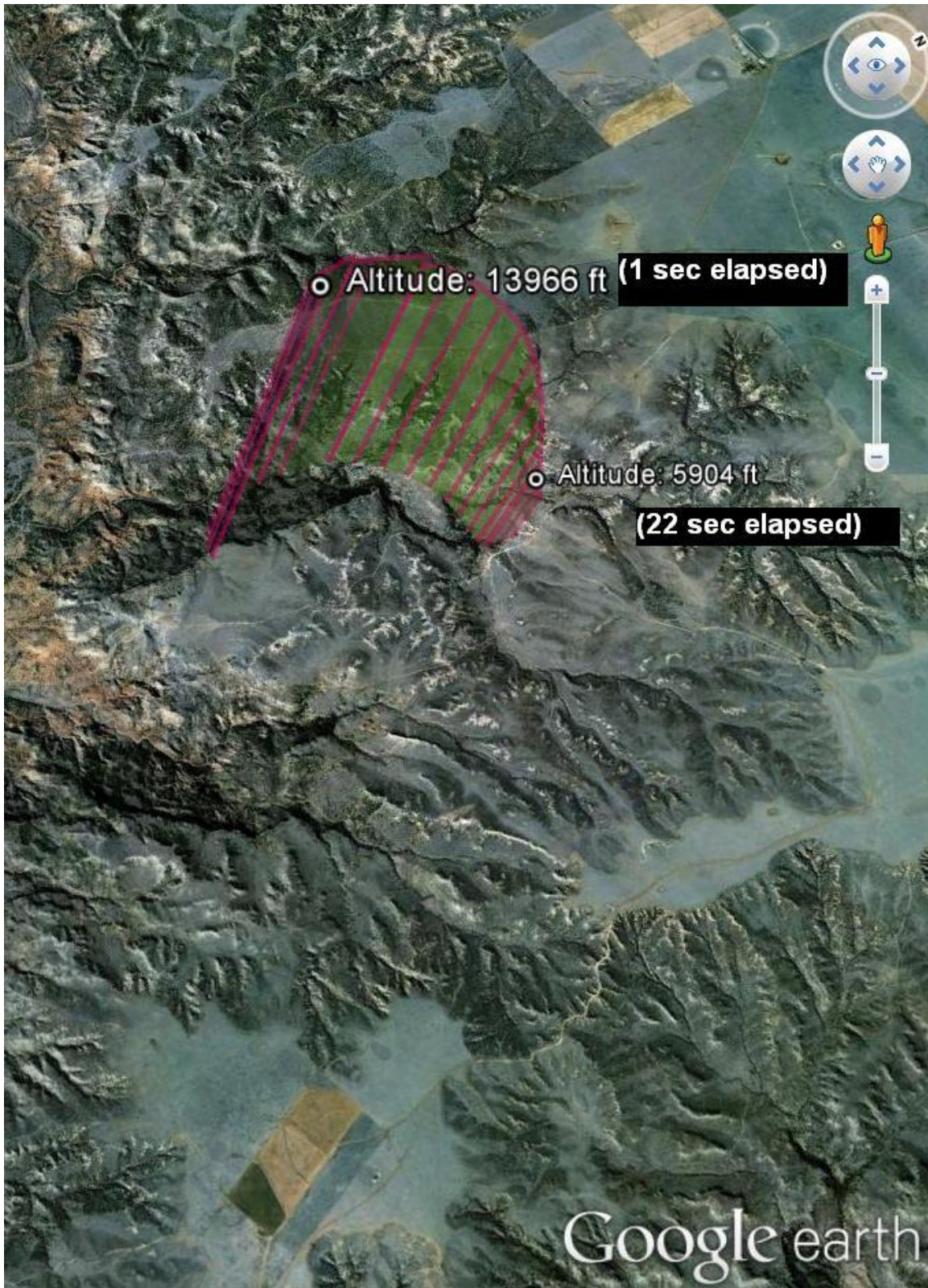
Figure 4. Google Earth overlay of EGPWS data from accident flight.
