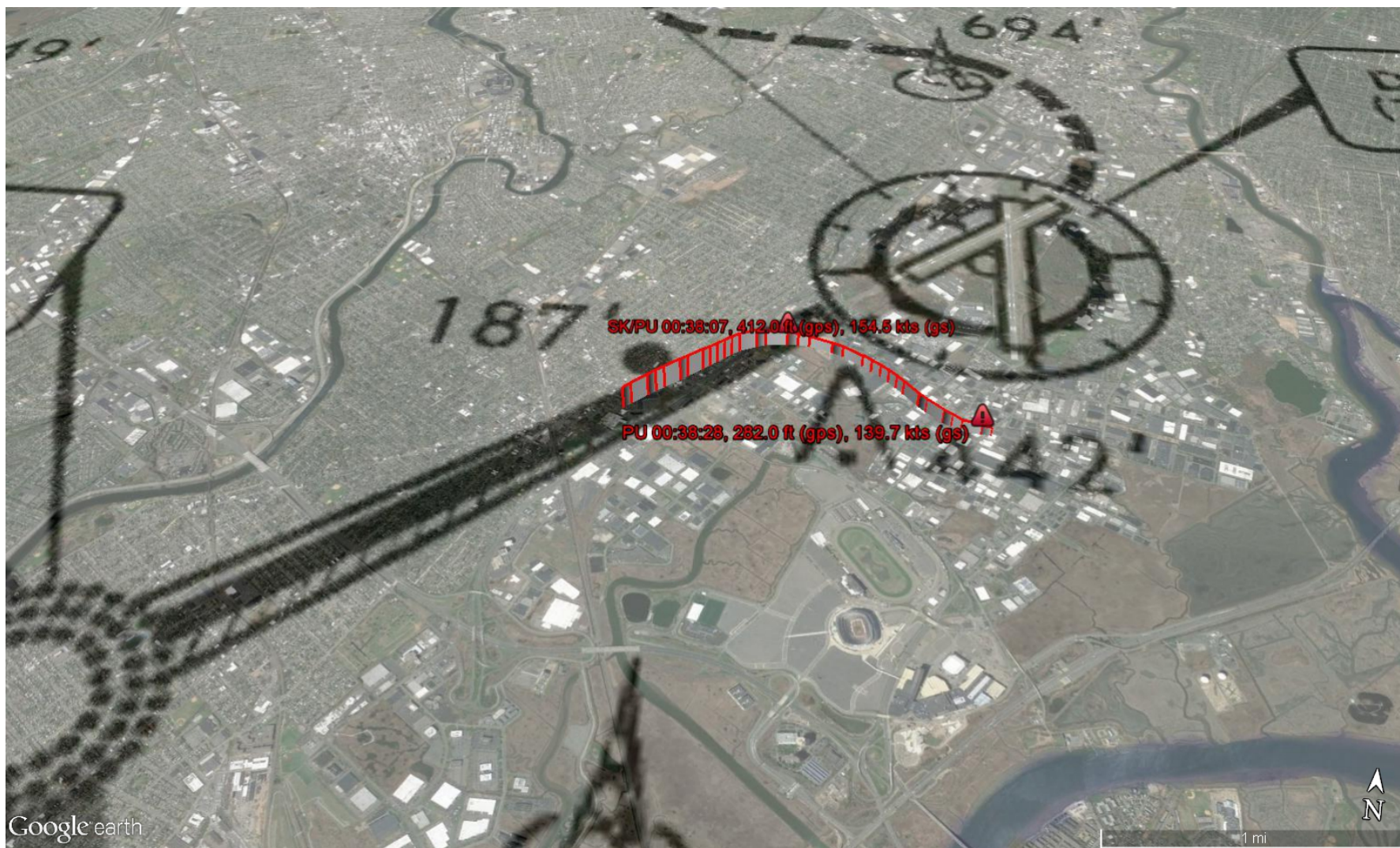
Figure 7. Accident leg 288, Jeppesen ILS 6 approach chart overlay, mid-level zoom (select points annotated).
