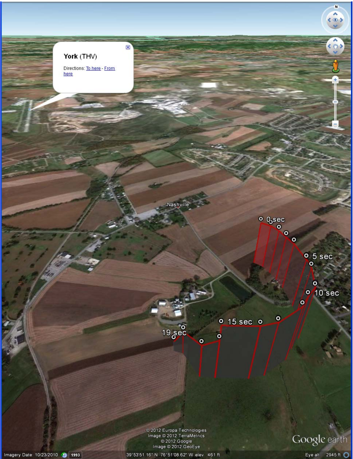
Plot 2 – EGPWS Data overlaid on a Google Earth terrain image using GPS altitude.
