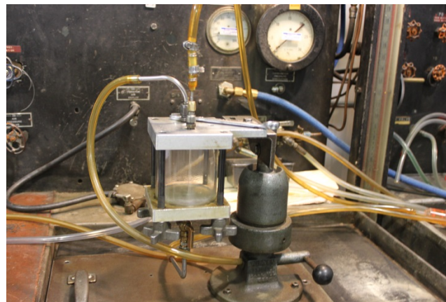
Figure 3: No. 1 fuel injector nozzle during testing.
