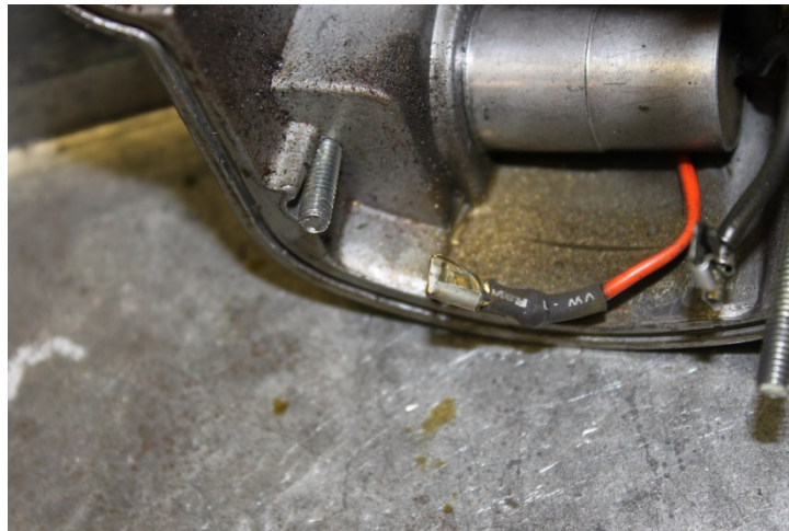
Figure 6: Broken push-on connector of the retard breaker switch lead.
