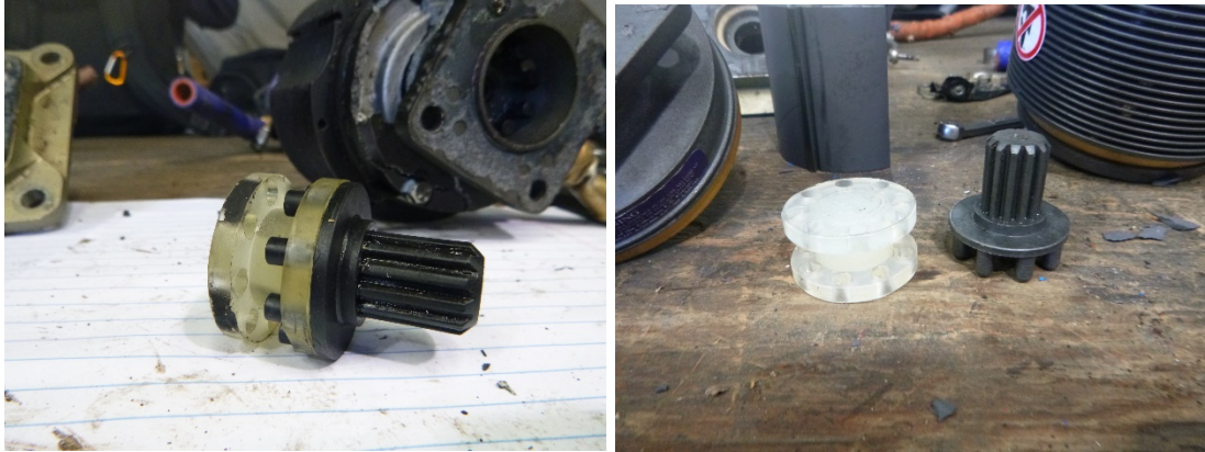
Photo 3 – Right and left vacuum pump plastic drive couplings
