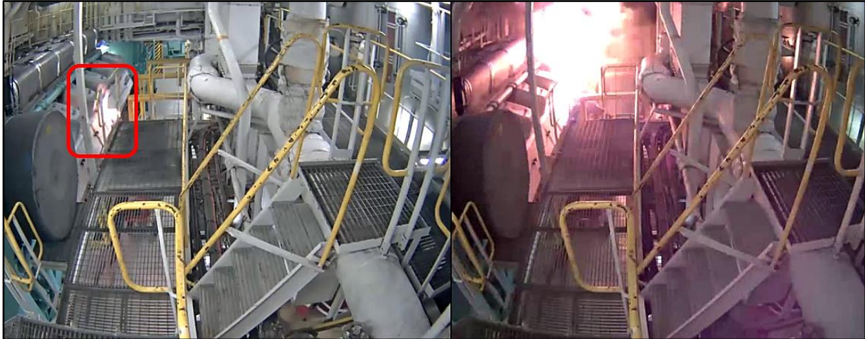
Images from the ship's closed-circuit television of DG 4 from forward looking aft. The red box on the left image highlights the first visual sign of open flame. The right image shows the same area less than 1 second later.
