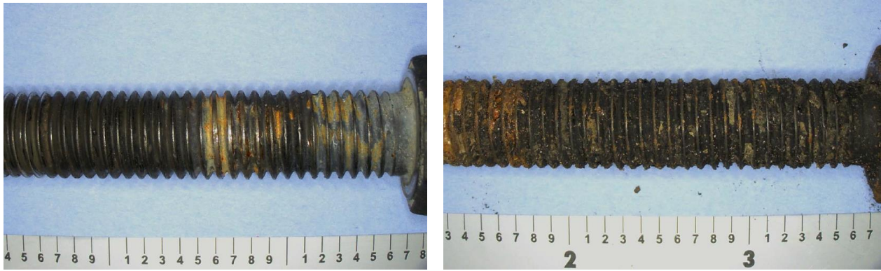
Left, the bolt found attached to the housing of the fuel-injection pump for cylinder A2. Discoloration and residue can be seen in some of the threads. Right, the bolt that was found detached.
